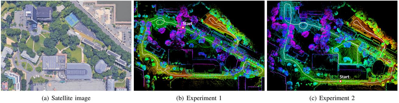
Fig. 6: LeGO-LOAM maps from experiments 1 and 2. The color variation in (c) indicates true elevation change. Since the robot’s initial position in experiment 1 is on a slope, the color variation in (b) does not represent true elevation change.
