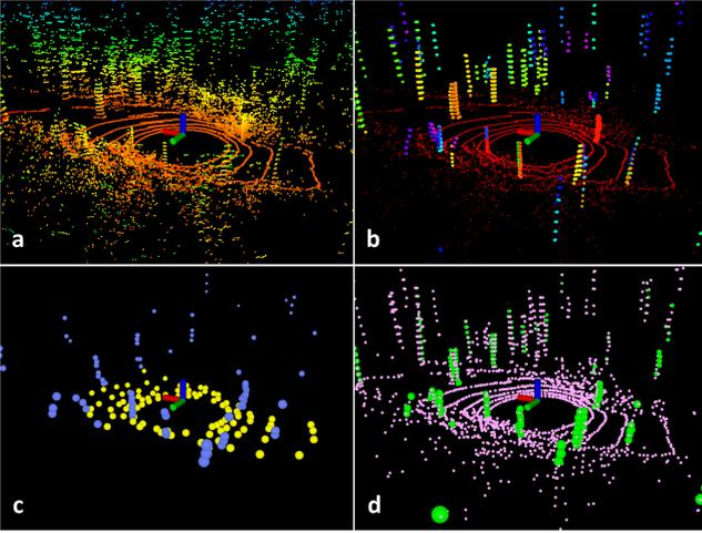
Fig. 2: Feature extraction process for a scan in noisy environment. The original point cloud is shown in (a). In (b), the red points are labeled as ground points. The rest of the points are the points that remain after segmentation. In (c), blue and yellow points indicate edge and planar features in  $F_e$  and  $F_p$ . In (d), the green and pink points represent edge and planar features in  $\mathbb{F}_e$  and  $\mathbb{F}_p$  respectively.
