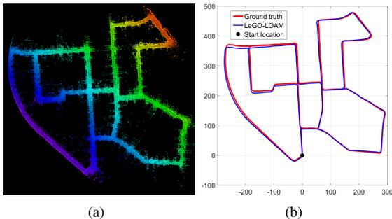
Fig. 10: LeGO-LOAM, KITTI dataset loop closure test, using the Jetson. Color variation indicates elevation change.
