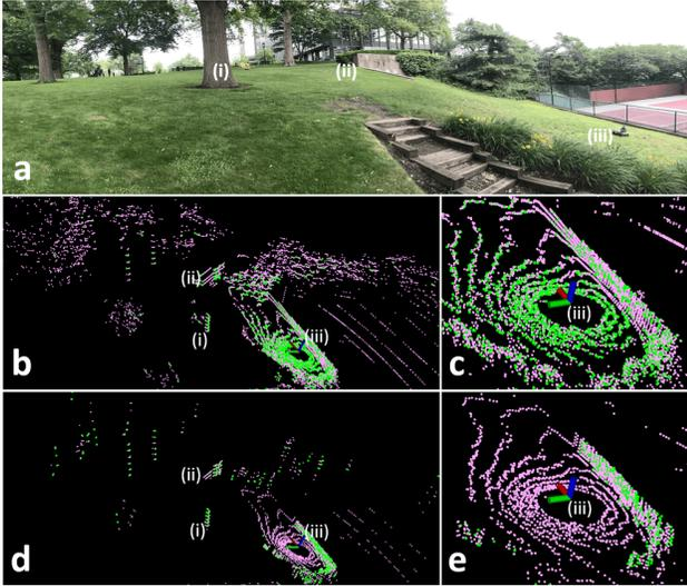
Fig. 4: Edge and planar features obtained from two different lidar odometry and mapping frameworks in an outdoor environment covered by vegetation. Edge and planar features are colored green and pink, respectively. The features obtained from LOAM are shown in (b) and (c). The features obtained from LeGO-LOAM are shown in (d) and (e). Label (i) indicates a tree, (ii) indicates a stone wall, and (iii) indicates the robot.
