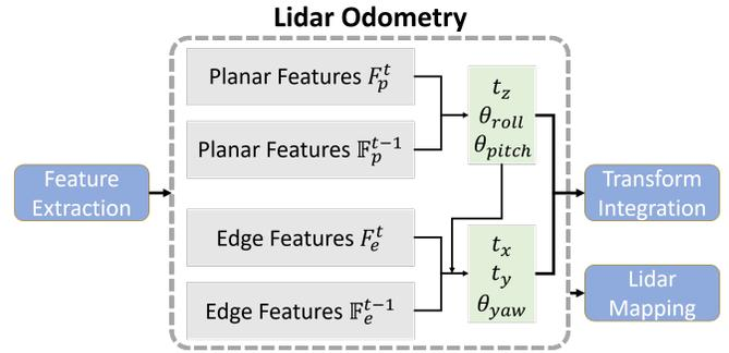
Fig. 3: Two-step optimization for the *lidar odometry* module.  $[t_z, \theta_{roll}, \theta_{pitch}]$  is first obtained by matching the planar features extracted from ground points.  $[t_x, t_y, \theta_{yaw}]$  are then estimated using the edge features extracted from segmented points while applying  $[t_z, \theta_{roll}, \theta_{pitch}]$  as constraints.
