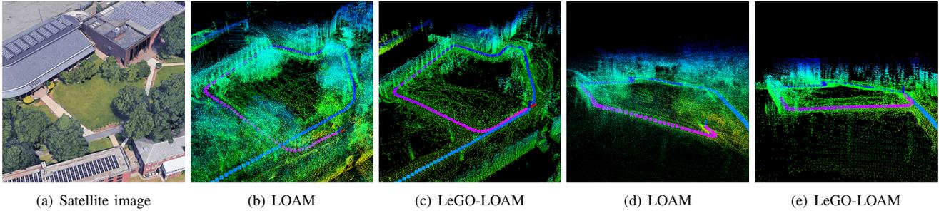
Fig. 7: A scenario where LOAM fails over a sidewalk crossing the Stevens campus in experiment 2 (the leftmost sidewalk in image (a) above). One end of the sidewalk is supported by features from a nearby building. The other end of the sidewalk is surrounded primarily by noisy objects, i.e., grass and trees. Without point cloud segmentation, unreliable edge and planar features will be extracted from such objects. Images (b) and (d) show that LOAM fails after passing over the sidewalk.
