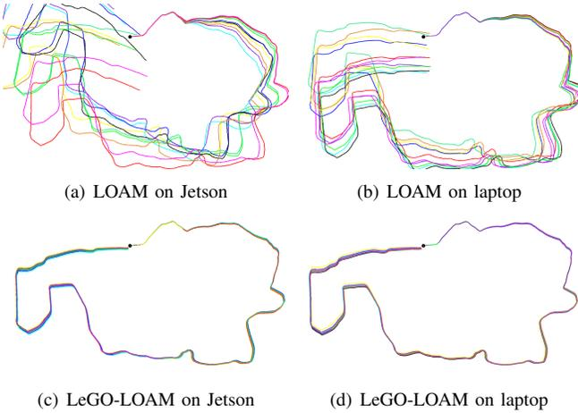
Fig. 9: Paths produced by LOAM and LeGO-LOAM across 10 trials, and 2 computers, with the experiment 3 dataset.
