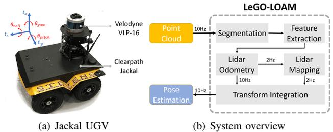
Fig. 1: Hardware and system overview of LeGO-LOAM.
