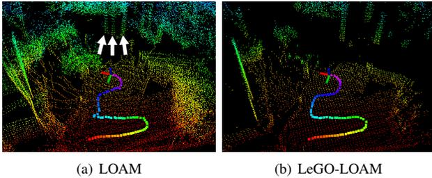
Fig. 5: Maps from both LOAM and LeGO-LOAM over the terrain shown in Fig. 4(a). The trees marked by white arrows in (a) represent the same tree.
