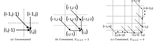
Fig. 2. DDTW local constraints that restrict the admissible paths to every location within the matrix: (a)  $C(i,j) = d(i,j) + \min(C(i-1,j-1),C(i,j-1),C(i-1,j))$  (b)  $C(i,j) = d(i,j) + \min(C(i-1,j-1),C(i-1,j-2) + d(i,j-1),C(i-2,j-1) + d(i-1,j))$  (c)  $C(i,j) = \min\left[\min_{1 \le r \le E_{MAX}} \left(C(i-1,j-r) + \sum_{j_1=j-(r-1)}^{j} d(i,j_1)\right), \min_{2 \le r \le E_{MAX}} \left(C(i-r,j-1) + \sum_{i_1=i-(r-1)}^{i} d(i_1,j)\right)\right]$
