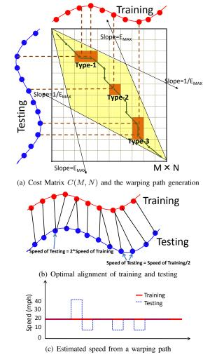
Fig. 3. Illustration of vehicular speed estimation from DDTW.
