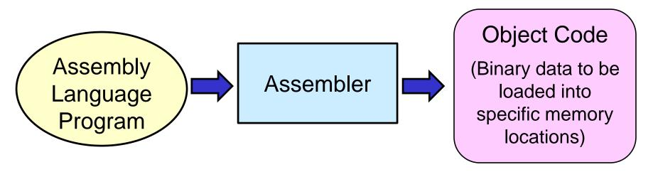
Assembler translates assembly code mnemonics & symbols into raw binary data to be loaded into microprocessor memory 3
