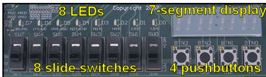
Figure 7: Nexys2 board I/O devices
