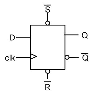
architecture DA1 of Dff is begin ff\_proc: **process** (clk,Rb,Sb) begin if Rb='0' then Q<='0' **after** 5ns; Qb<='1' after 5ns; elsif Sb='0' then Q<='1' **after** 5ns; Qb<='0' after 5ns; elsif clk'event and clk='1' then Q<=D after 7 ns; Qb<= not D after 7 ns; end if; end process ff\_proc; end architecture DA1;
