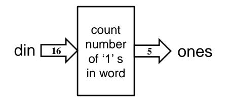
architecture A1 of count1s is begin p1: process (din) variable count: integer; begin count:=0; for i in 0 to 15 loop if din(i)='1' then count:= count+1; end if; end loop; ones<=conv\_std\_logic\_vector(count,5) after 5ns; end process; end A1;
