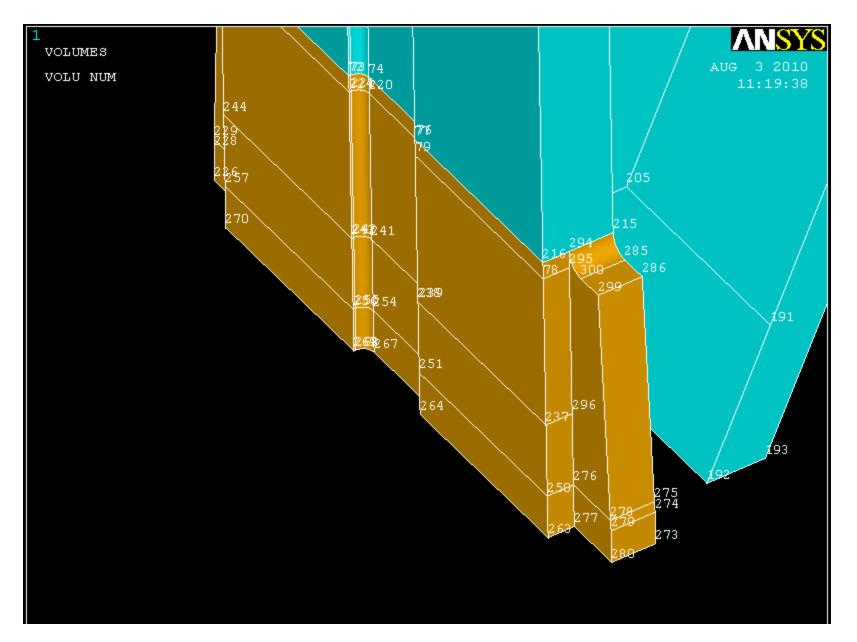
To create matching keypoints on the large volume take the top face of the smaller volume shown below and extrude it -.5 in the z direction (ANSYS will give you an option to choose between two areas, pick the area with the higher number). Add this new volume to the large volume (be careful not to select the volume we created in the previous step).
