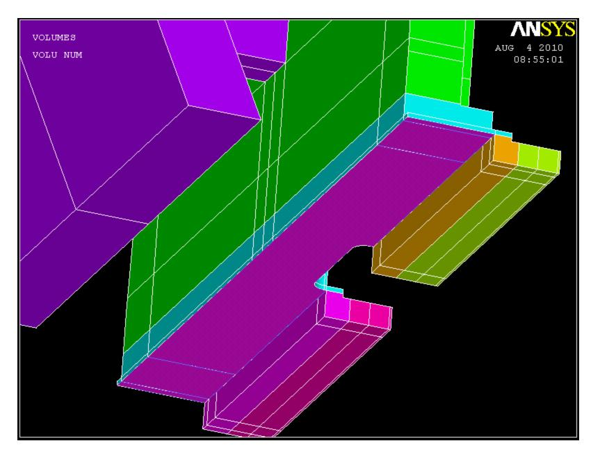
To create the corresponding keypoints, extrude the highlighted faces by 1.875 in the y direction
