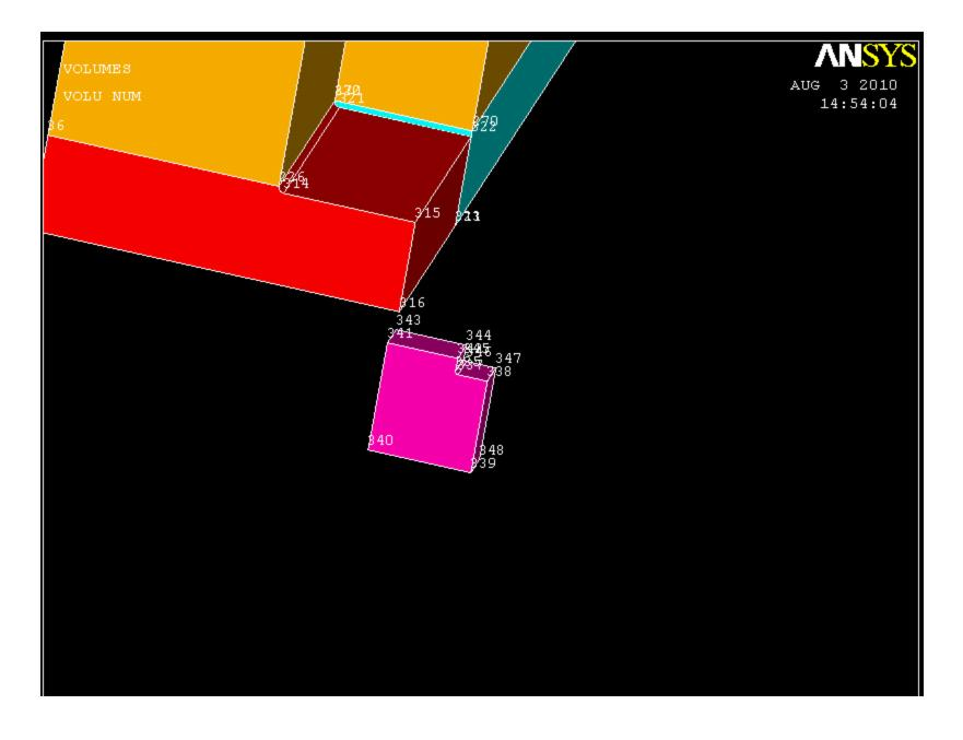
Extrude the rightmost area of the new volume .5 in the y direction
