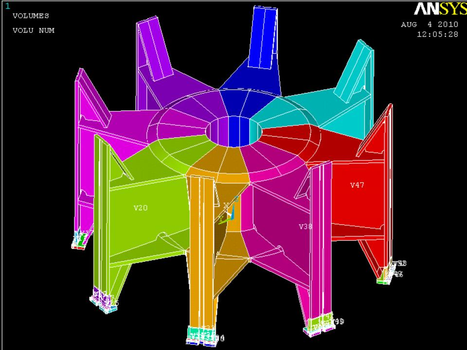
For the sake of having a final model that will be able to be analyzed, merge your keypoints (Preprocessor >> Numbering Controls >> Merge Items >> Keypoints) compress your keypoint numbers (Numbering Controls >> Compress Items), again. Compressing the volumes won't do anything this time because ANSYS automatically created everything for you.
