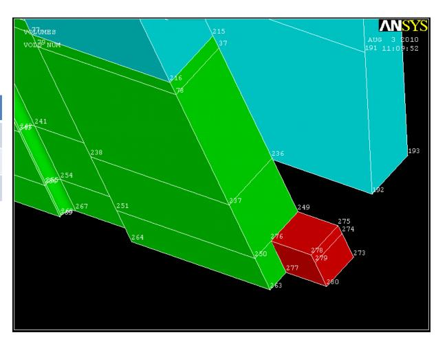
Create 3 keypoints. Using the first two and the keypoint that intersects both volumes create and arc of radius .5 (the first keypoint listed and the keypoint on the body are the end points and the second keypoint listed is the center). Connect the last keypoint listed and the to the end of the arc and to the volume below it using straight lines, then create an area by lines as shown below. Note: the vertical line is actually 3 lines vertical lines when you are selecting.
