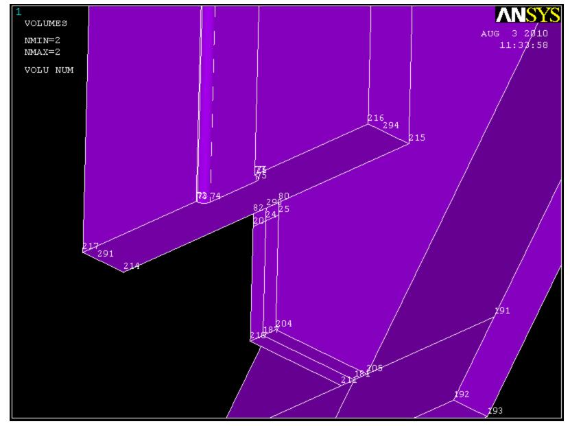
Select the bottom face of the smaller volume (shown below) and extrude it -.53125 in the z direction, keep it separate for now.
