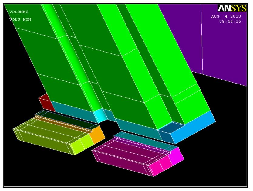
Extrude the three highlighted faces shown below by -.1 in the z direction.
