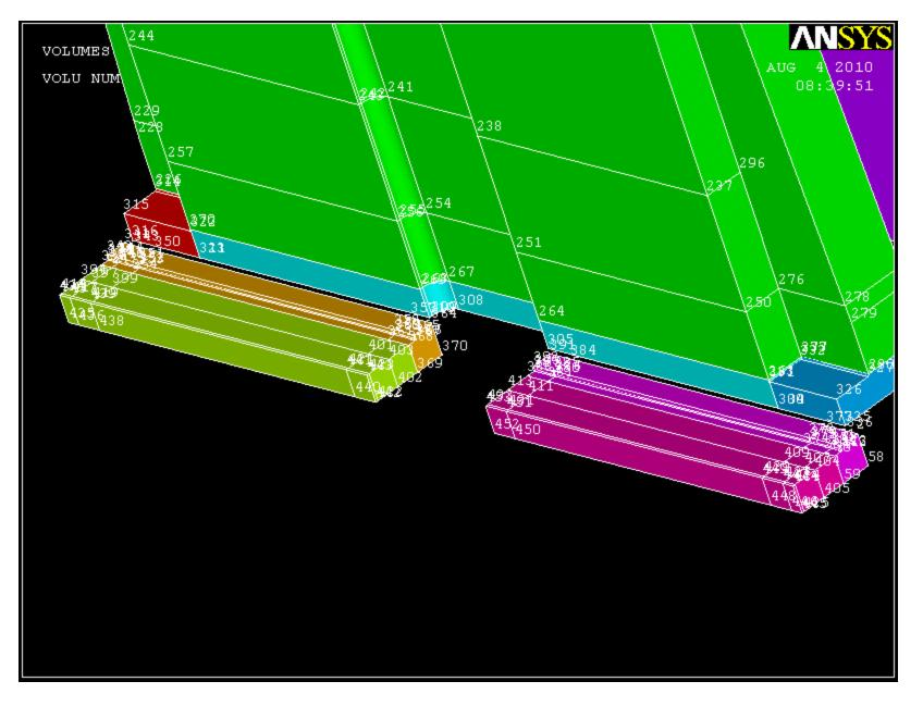
Extrude the eight highlighted faces shown below by .1 in the z direction. (Keypoint numbering has been turned off for now *(Plot Controls >> Numbering)*)
