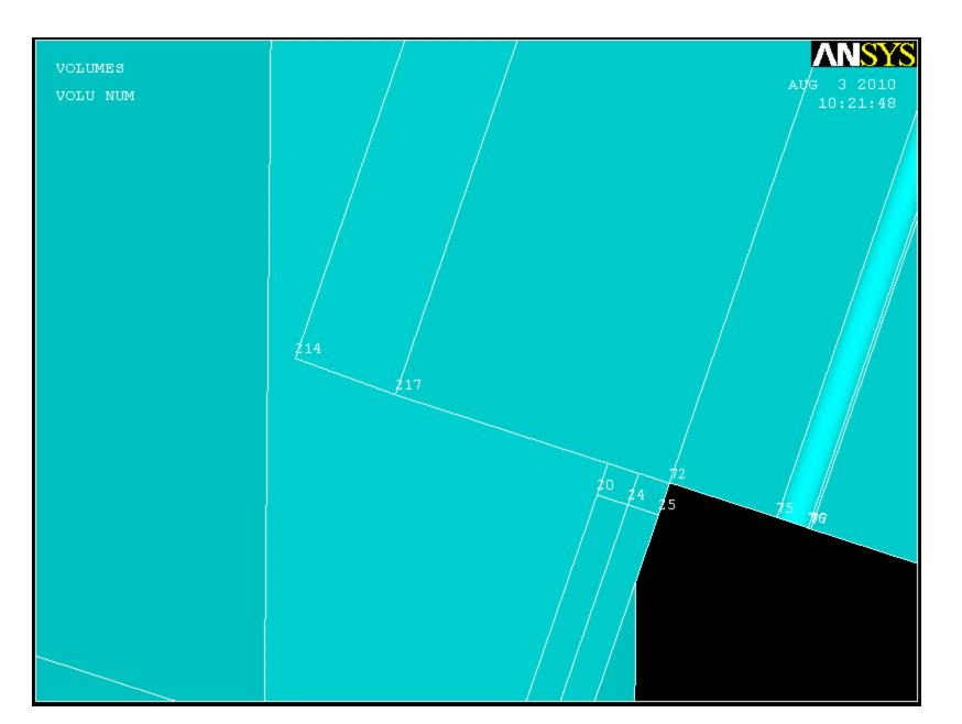
Now, extrude that same face -.5 in the z direction, but leave it as a separate volume. Now the keypoints match up on both volumes, so the model can transfer loads properly.
