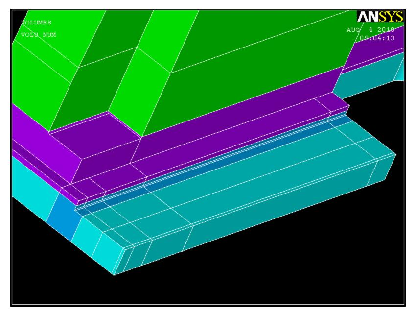
To create the corresponding keypoints, extrude the highlighted faces by -1.875 in the y direction
