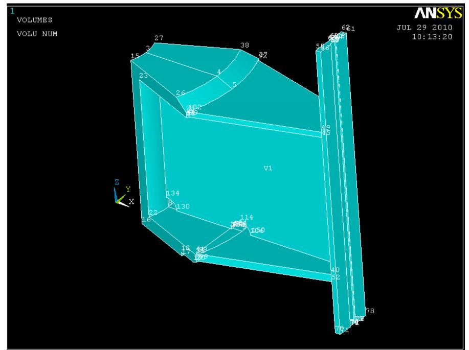
Create 5 new keypoints and connect them by lines – a sixth keypoint will be needed it is already on the model at 93.5,0,90. Then create an area by lines from these 6 lines.
