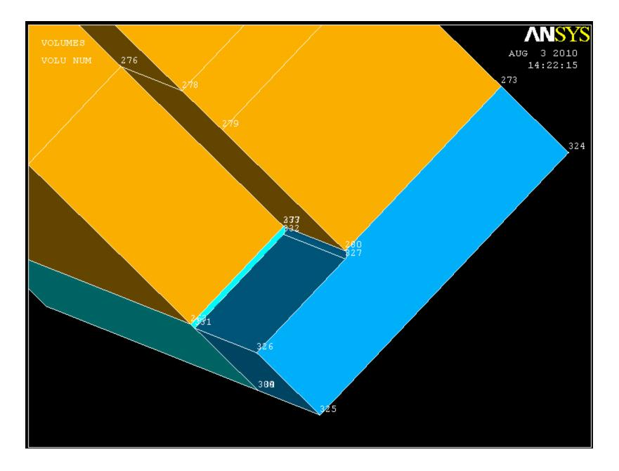
Create 8 new keypoints. The first three are used for an arc of radius .015625 (the first two are the endpoints and the third is the center point. Connect the rest with straight lines as shown below and create an area by lines as shown below.
