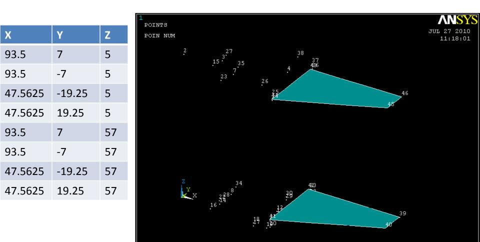
Now extrude the areas the appropriate distances - 2 for the top and -2.75 for the bottom, both in the z direction *(Operate >> Extrude >> Areas >> by XYZ offset).* To plot your volumes you can either type "vplot" into the command line, or click *(plot >> volumes)*.
