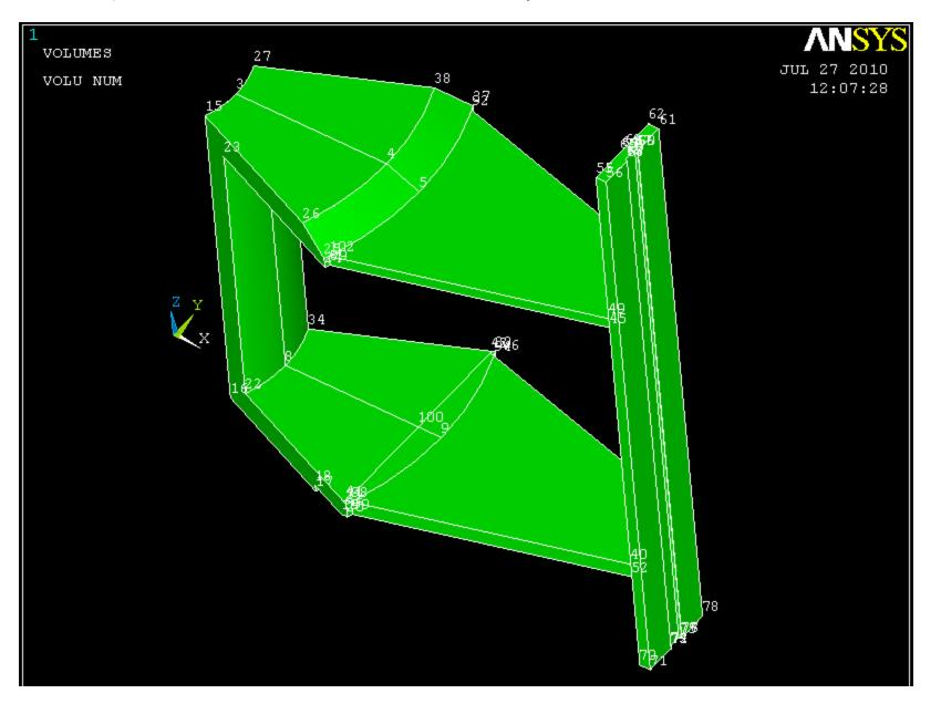
Select the two inner faces of the spider arm as shown, and extrude by XYZ offset, -75 in the X direction. Add these two volumes together, but keep it separate from the big volume.
