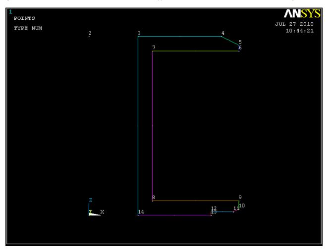
Create the area to be extruded (creates > area > arbitrary > by lines), when done, click okay to exit the box. Select the lines in order – start at one line and then click the one with the coincident endpoint, until you complete a closed area (ANSYS is dumb and crossing lines and keypoints confuses it). Your area should look like the one below.
