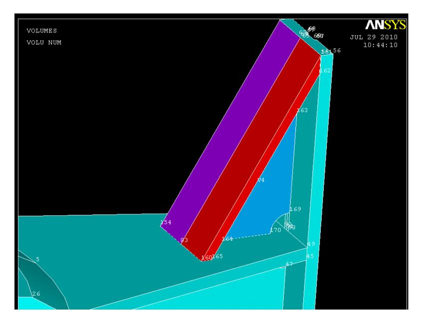
Create 6 new keypoints. Connect them with 6 new lines as we did in the last set. Then create an area by lines. The arcs and extra lines should be used for reference for the next slide's instructions – in other words I forgot to take a screenshot.
