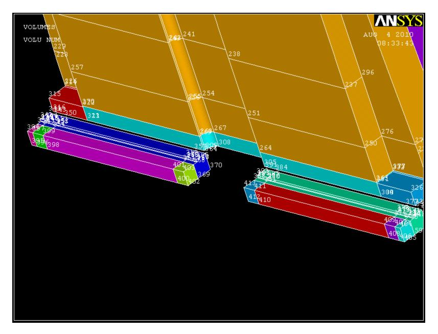
Select the front faces of the new volumes, and extrude them .45 in the x direction again (we are creating keypoints to be used for the model with the blocks later).
