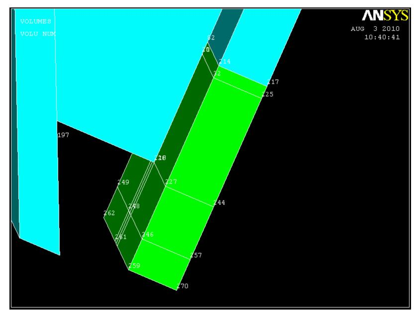
Go to *(Preprocessor >> Numbering Controls >> Merge Items)* and select keypoints and hit okay. This will merge the keypoints that are at the same location, joining the two volumes while keeping them separate, and making for simpler geometry creation as we continue to build.
