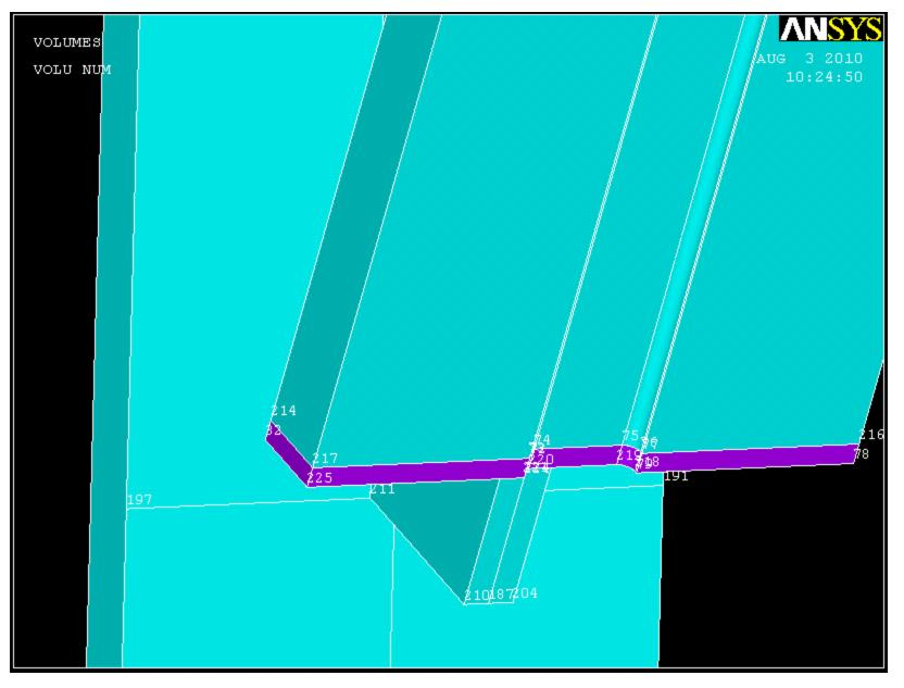
Now, extrude the bottom area of the new volume -4.5 in the z direction (again to match keypoints).
