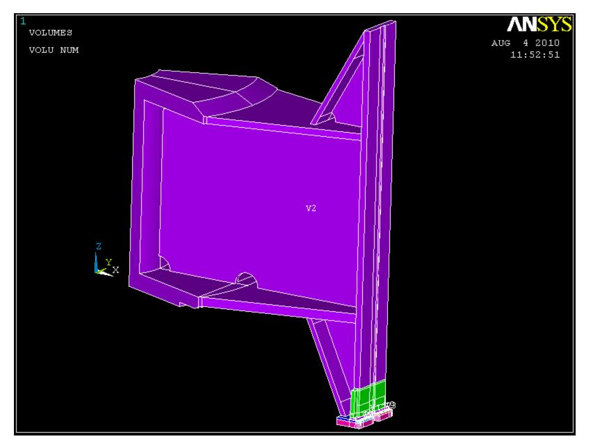
Switch to a cylindrical coordinate system, by typing "csys,1" in the command line ("csys,0" will bring back cartesian coordinates). Now, we want to create full symmetry, so go to *(Modeling >> Copy >> Volumes)* hit pick all, and type 8 in the number of copies box, as well as 45 in the Y direction because we want a full 360 model from an 8<sup>th</sup> model.
