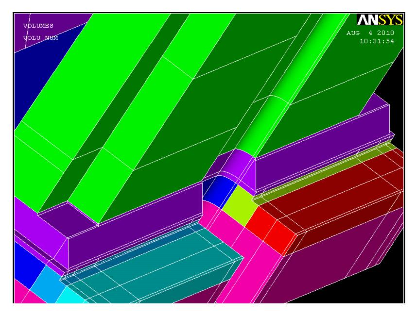
Merge your keypoints (*Preprocessor >> Numbering Controls >> Merge Items >> Keypoints*) as well as compress your volume and keypoint numbers (*Numbering Controls >> Compress Items*)
