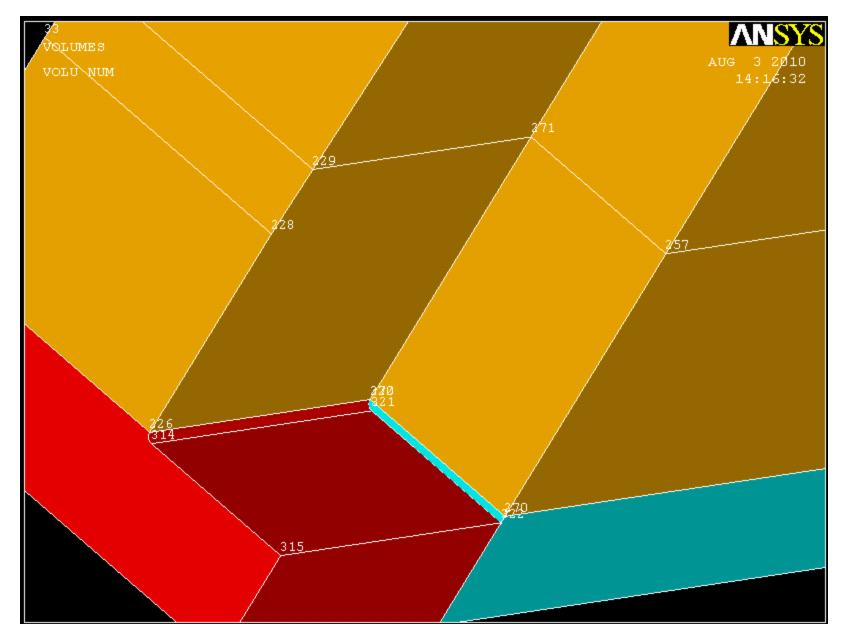
Create 5 new keypoints. Using the first (endpoint) and second (center point) keypoints, and the right most point of the second volume, create an arc of radius .03125. Connect the rest of the new keypoints with straight lines to form the area below.
