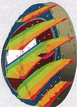
Temperature contours at the Tsherepovets Arena, showing stratification of several parameters during an ice hockey game in summer conditions with displacement ventilation.
