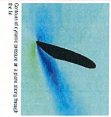
Patterns, covered by vorticity magnitude, illustrate the strong recirculation that occurs on the downwind side of the fin.
