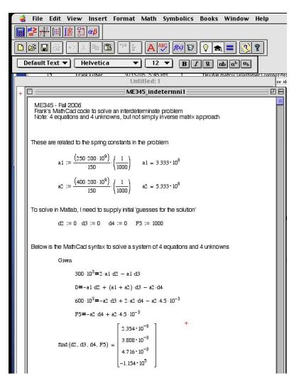
Note: to solve via matrix multiplication (inverse), you can rewrite the equation such that all unknowns are on one side of the equation. Doing this here (and using the fact that d1 = 0, d5 = 4.5e-3 m, and a1 and a2 are the element stiffness terms for the thin and thick sections, respectively), you would get:
