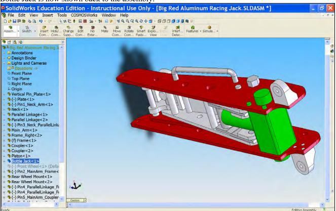
31) Now, we will define a contact type to the assembly. Expand the tree item labeled **Connections** then **Component Contacts** and right click on **Global Contact** and click Edit Definition
