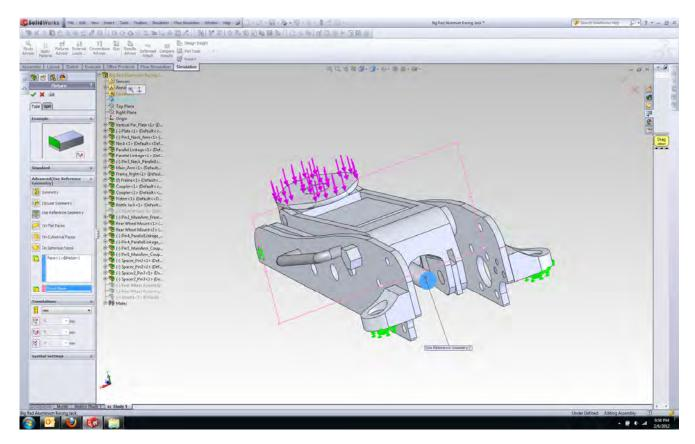
28) We have completed applying restraints to the assembly. Now, we can show the Bottle Jack back to the assembly.
