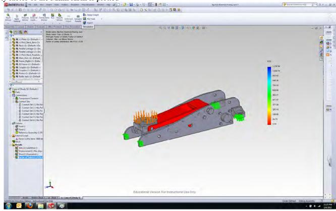
89) This floor jack assembly was modeled with a parameterized function that allows the user to modify the geometry of certain component and having the SolidWorks to automatically change the geometry of the other components associated with the component which its geometry was manually modified. For instance, if you change the diameter of a pin, the hole in which the pin is inserted into is automatically modified with respect to the change in the pin diameter.
