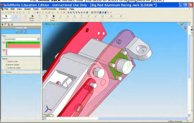
69) For Faces for Target, select the surface of the Left Frame as shown in the picture below. Under Options, select Node to Surface. Click OK. (Note: The Left Frame surface that you need to select is highlighted in pink.)
