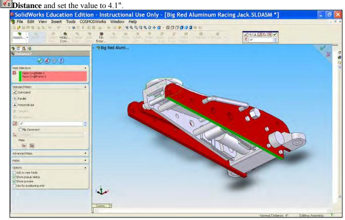
8) The top face of the plate and the bottom face of the frame are now 4" from each other. Now we will use SolidWorks to analyze the stress on the floor jack assembly when the load is applied. Click on the Simulation tab
