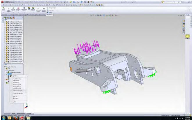
25) For Faces, Edges, Vertices for Restraint, click on the end face of the piston as shown in the picture.
