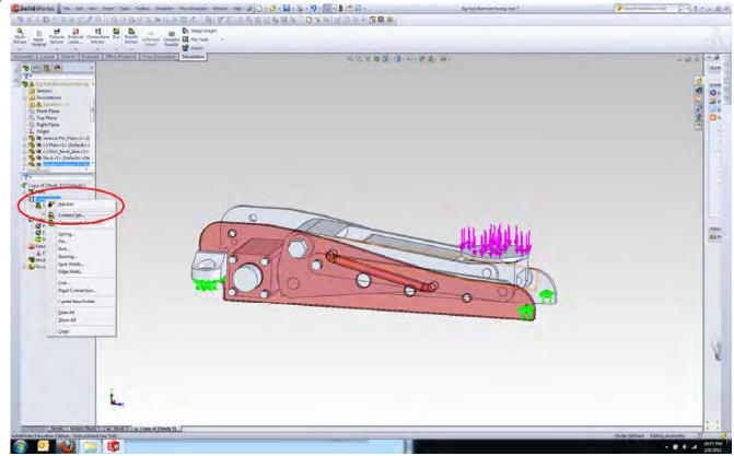
56) For **Faces, Edges, Vertices for Source,** select the face of **Bottle Jack** as shown in picture below. (Note: The **Bottle Jack** surface that you need to select is highlighted in green.)
