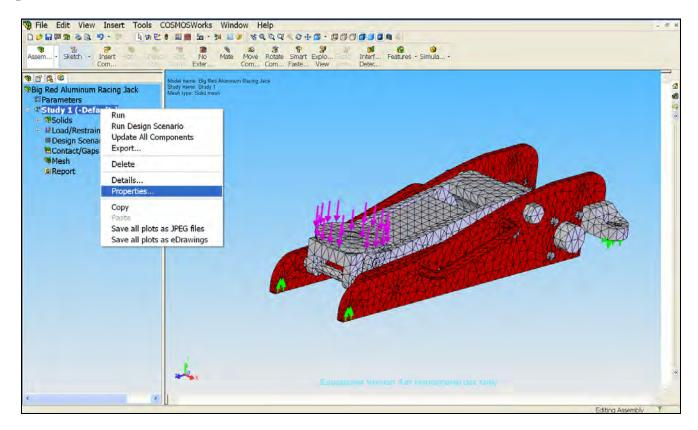
37) Select **Direct sparse** as a solver and click **OK**. Using Direct sparse as a solver will minimize the time to run the analysis and it also gives more accurate results. However, the downside of using this solver is that it uses too much RAM space which will cause the computer to run slow.
