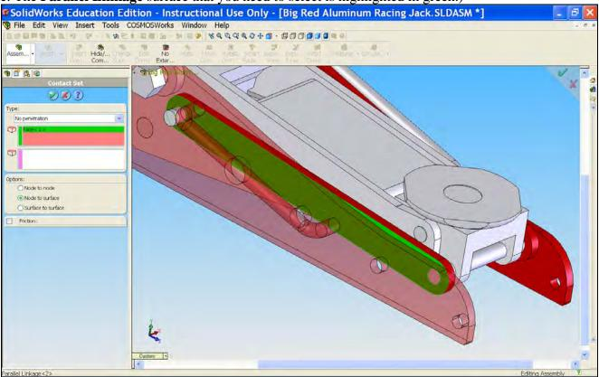
51) For Faces for Target, select the surface of the **Right Frame** as shown in the picture below. Under **Type**, select **No Penetration**. Click **OK**. (Note: The **Right Frame** surface that you need to select is highlighted in pink.)
