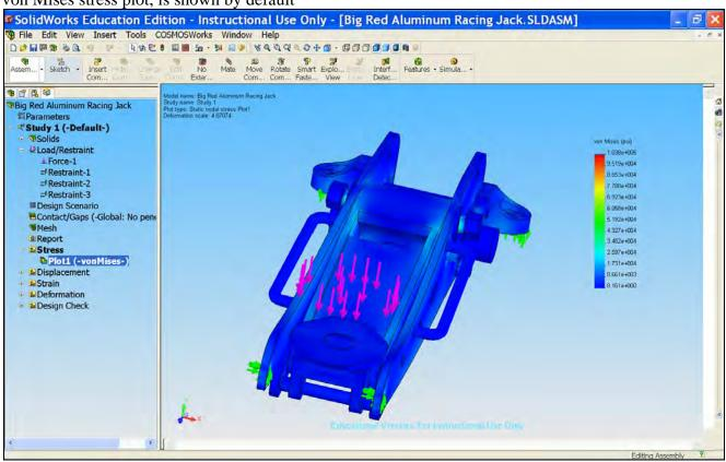
42) To better understand how the parts deform under loading, we can use an animation function to show us the stress and deformation of the assembly over a period of time. Go to **Simulation** menu on top, then go to **Result Tools** and select **Animate**.
