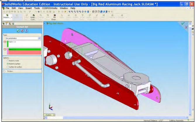
70) We have completed defining gaps to avoid interference of the parts with the left frame. We can now change the transparency of the left frame back to normal. Put the mouse pointer anywhere on left frame surface and right-
