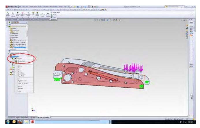
**Faces, Edges, Vertices for Source,** select the face of **Parallel Linkage** as shown in picture below. 62) For (Note: The Parallel Linkage surface that you need to select is highlighted in green.)
