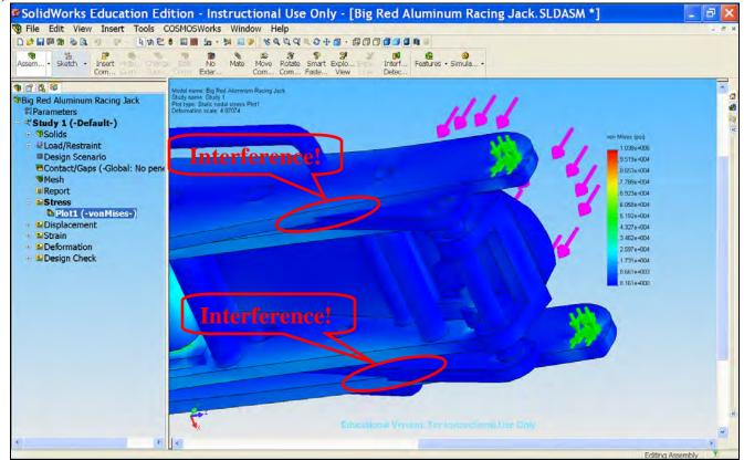
47) To fix the interference problem, we need to further define the contact or gaps for the assembly. First, put the mouse pointer anywhere on right frame surface and right-click it. Then, select Change Transparency.
