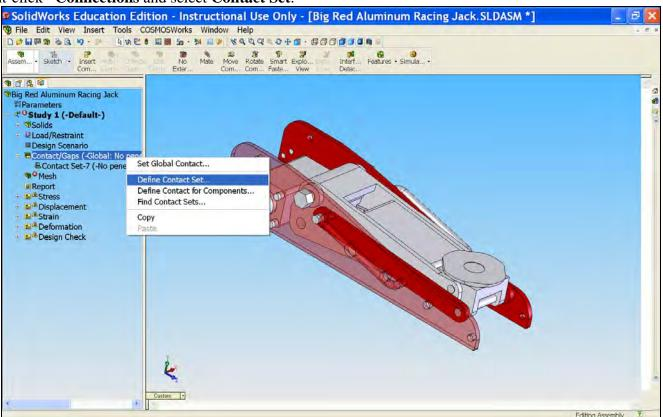
53) For Faces, Edges, Vertices for Source, select the face of Spacer Pin2<2> as shown in picture below. (Note: The Spacer Pin2<2> surface that you need to select is highlighted in green.)
