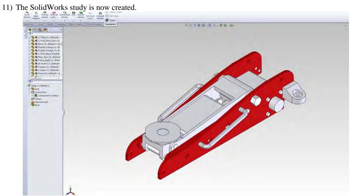
12) Now, we need to assign material for the floor jack assembly. Under Study1, right-click Parts and select Apply Material to All.
