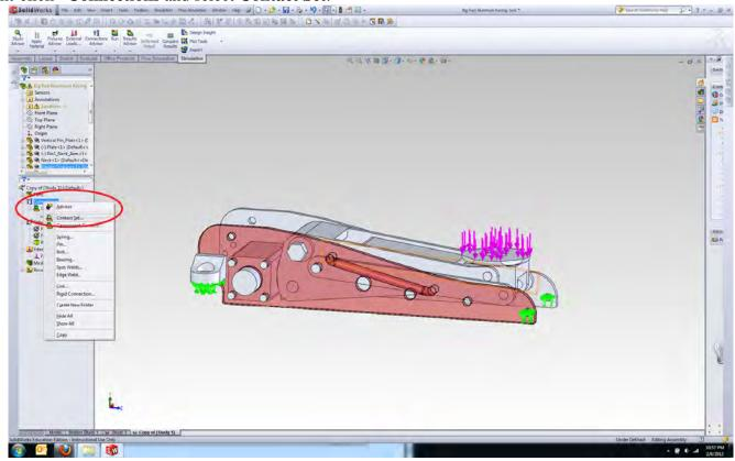
50) For Faces, Edges, Vertices for Source, select the face of Parallel Linkage as shown in picture below. (Note: The Parallel Linkage surface that you need to select is highlighted in green.)
