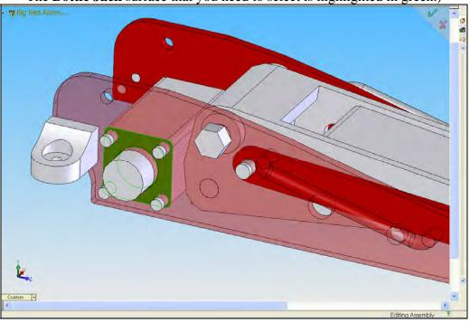
57) For Faces for Target, select the surface of the Right Frame as shown in the picture below.
