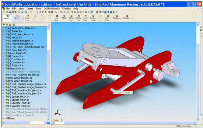
6) Now, we will define a distance between the plate, which supports the load from a car, and the ground. For this
