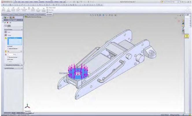
17) Change the Units to English (IPS). Under Force, select normal to direction and set 3000 as the magnitude of force. Check that force is pointing downward.
