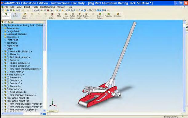
2) First of all, we need to suppress the front wheel, rear wheel assemblies and handle. To suppress all of those parts simultaneously, left-click **Front Wheel** and ctrl+left-click **Rear Wheel Assembly** <1>, <2> and **Handle**.
