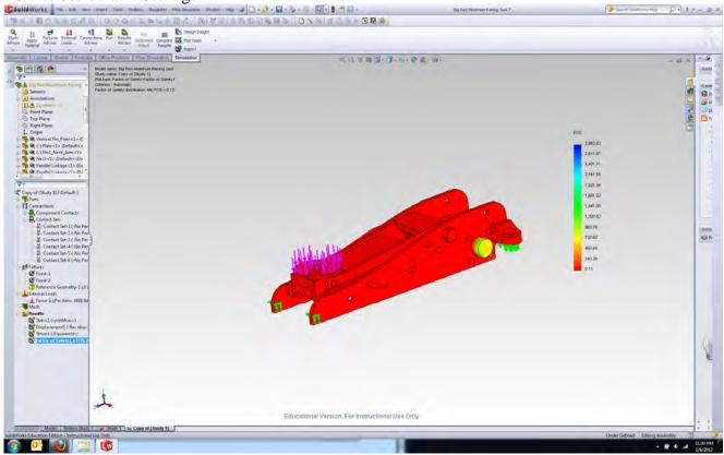
86) Now, let us find out the safety factor of individual component. Since the **Main Arm** is one of the most important parts that determine how much load the floor jack can support, let us plot the safety factor of the **Main Arm**. Right-click **Factory of Saftey** and **Edit Definition**.
