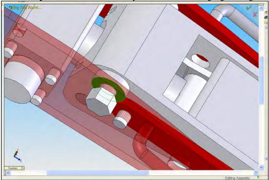
54) For Faces for Target, select the surface of the **Right Frame** as shown in the picture below. Under **Options**, select **Node to Surface**. Click **OK**. (Note: The **Right Frame** surface that you need to select is highlighted in pink.)
