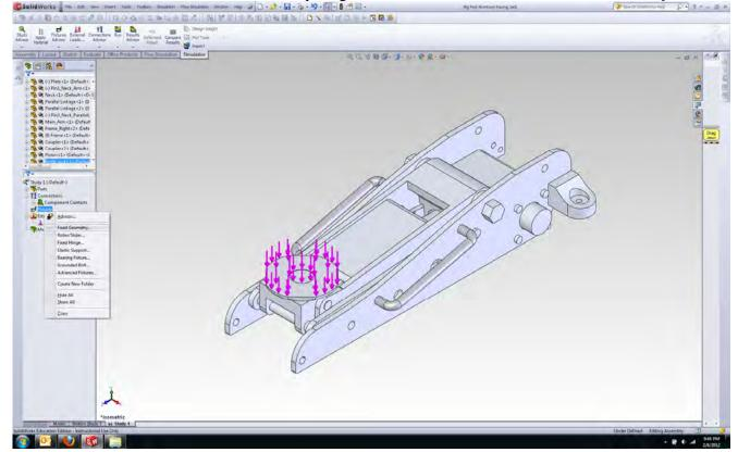
19) For Faces, Edges, Vertices for Constraint, select two upper half of the cylinder where the shaft for the front wheel is mounted. Refer to the picture below.
