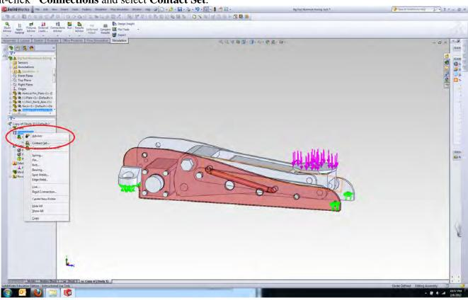
65) For Faces, Edges, Vertices for Source, select the face of Spacer Pin2<1> as shown in picture below. (Note: The Spacer Pin2<1> surface that you need to select is highlighted in green.)
