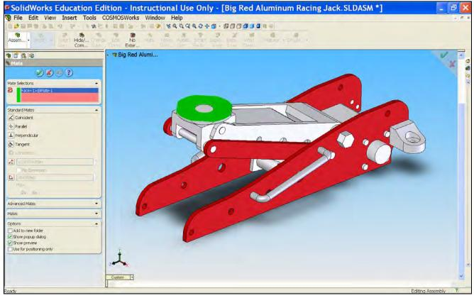
7) Second, select the bottom face of the frame as shown in the screen shot below. Under **Standard Mates**, click on
