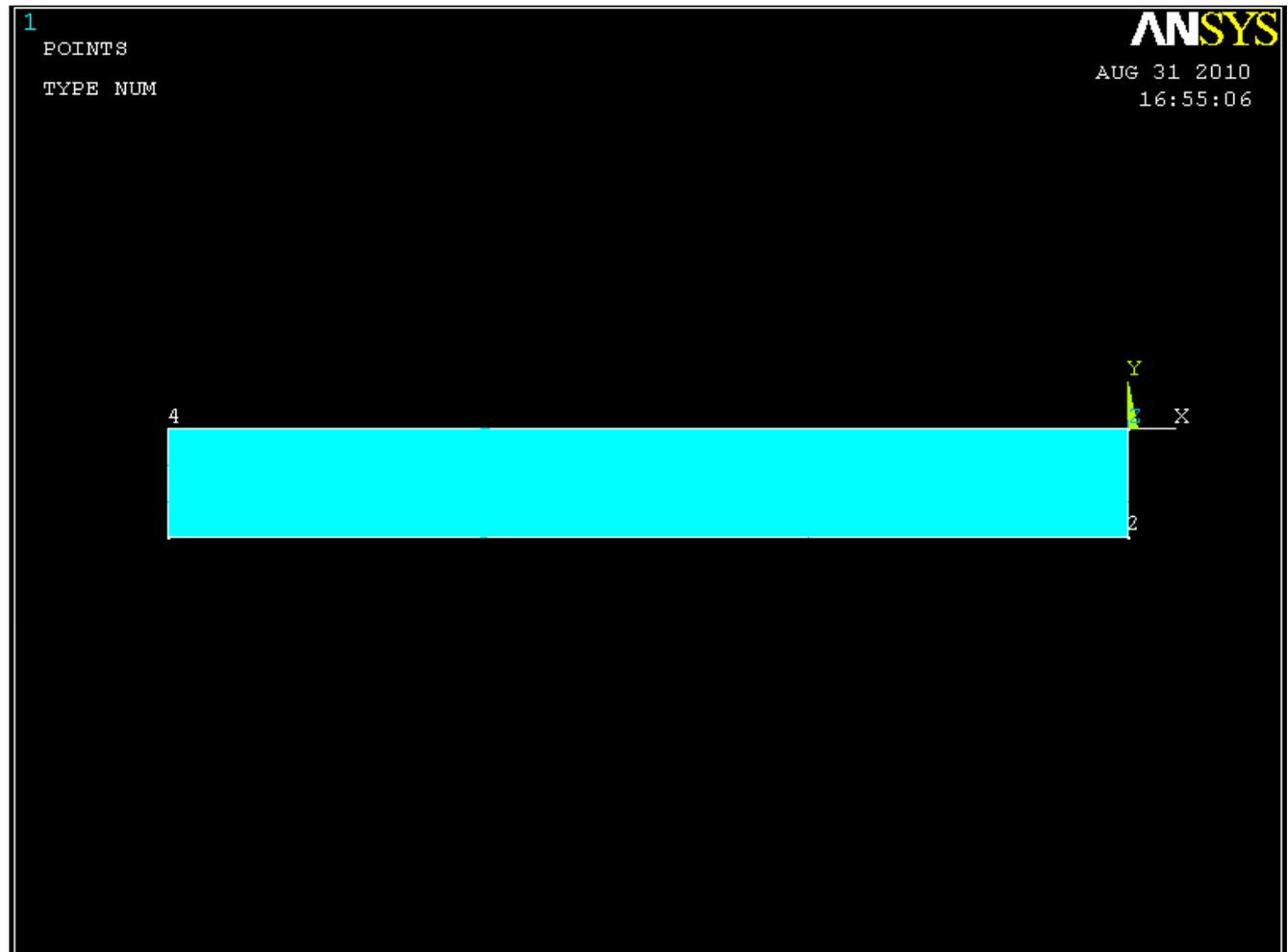
Extrude this area by xyz offset (**operate >> extrude >> areas >> by xyz offset**), -2.03 in the Z direction
