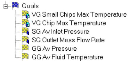
In this tutorial the engineering goals are set to determine the maximum temperature of the heat generating components, the temperature rise of the air and the pressure drop and mass flow rate through the enclosure.
