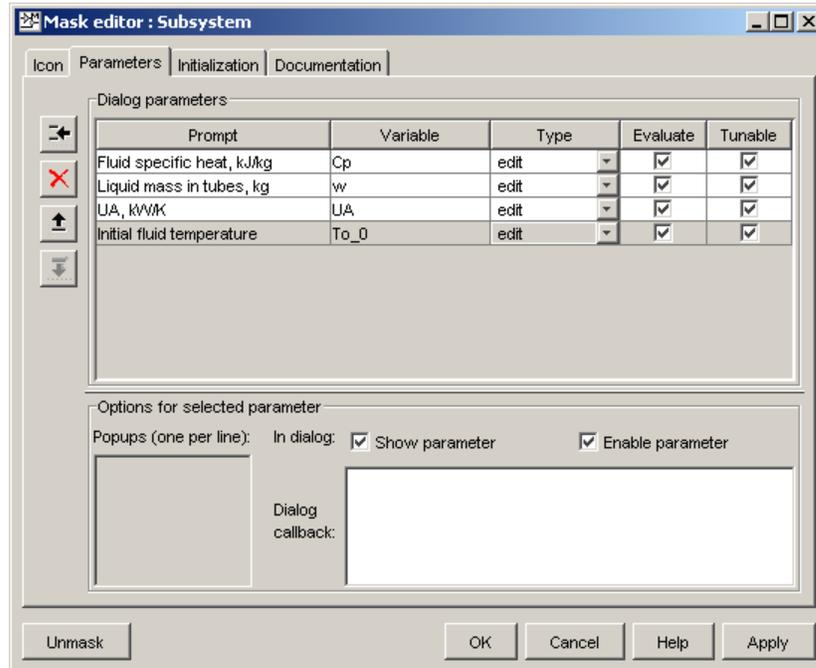
Figure 24 Mask editor with block parameters defined
