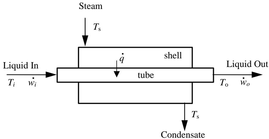
Figure 1 Shell-and-tube heat exchanger schematic
