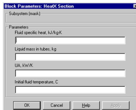
Figure 25 User interface for the HeatX Section block
