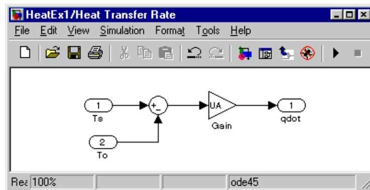
Figure 18 Heat transfer rate subsystem
