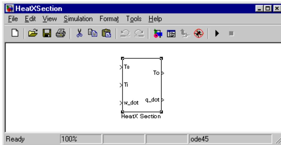
Figure 20 Block to model a heat exchanger section
