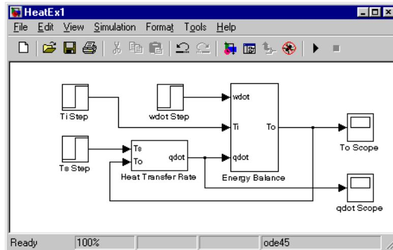
Figure 17 Heat exchanger model -- main window
