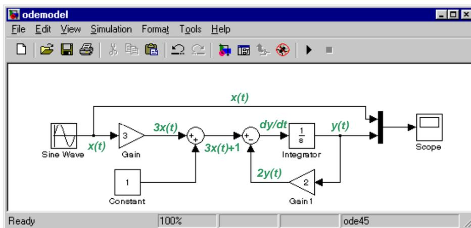
Figure 10 Simulink model of a linear, first-order ODE
