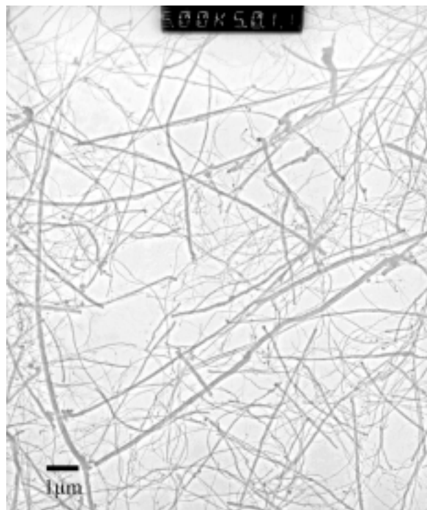
Fig. 1: TEM image of MWNTs dispersed in NMP prior to composite fabrication.
