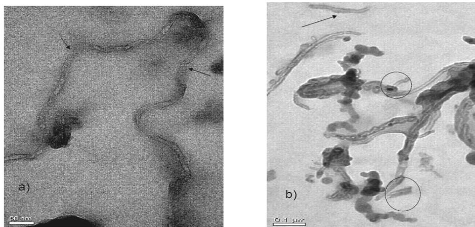
**Figure 2.** TEM images of functionalized carbon nanotubes. Arrows indicate where nanotubes appear damaged by the functionalization process. (Scale bars: left = 50 nm, right = 100 nm.)
