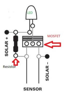
The above sensor relies on relatively inexpensive parts. The most expensive part is the MOSFET which retails for under three dollars at Radio Shack. The valued added in the project comes from interfacing the sensor with a WI-FI transmitter to communicate the soil status. The product is further enhanced by enclosing it in a brushed aluminum case which is light weight and corrosion resistant.
