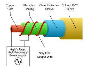
Now to make the EL wire glow, an AC voltage needs to be applied to the inner and outer copper wires. This voltage is typically between 90V to 200VRMS at a frequency in the low kilohertz. The brightness of the EL wire depends highly on the power applied, however it would be possible to power EL wire directly with the standard 120VAC, 60Hz line power.
