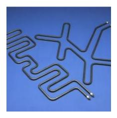
A tubular heating element acts as an elongated resistor formed into some shape to fit an application. Current is applied from one end of the tube to the other at one of several types of terminating ends. Terminating end types include "threaded stud, threaded bulk head, screw lug, quick disconnect spade, ceramic to metal hermetic, molded rubber lead, [and] conventional lead-wire terminal assembly" (Durex Industries).
