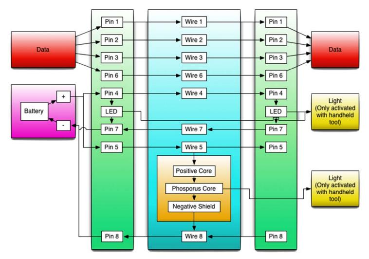
Starting with a fundamental function of our patch panel, data will be passed over pins 1,2,3,6 of the patch panel untouched by our added components. This is to ensure any impedance our LEDs may add will not corrupt the data.
