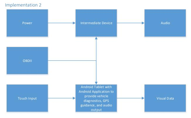
In this block diagram implementation, the power and audio connections will have an intermediate piece of hardware to connect into. This will allow the power and audio to always be connected into this intermediate device allowing for easy removal of the android tablet. This makes it much easier to install as well. The OBDII will still connect via Bluetooth and touch input and visual data output will still be interfaced through the touch screen on the tablet.
