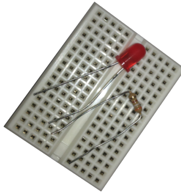
Breadboard, 330Ω resistor, and an LED
