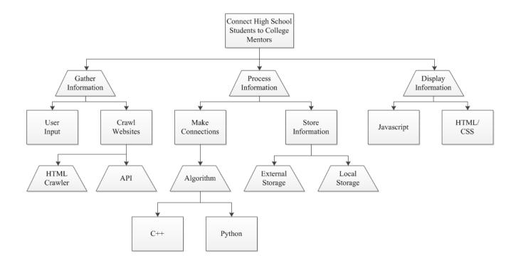
The function-means tree analyzes the various functions and required means of execution in order to satisfy the needs of the system. For the group's web service, the three primary means to support the function of the system are to gather information, process information, and display information.
