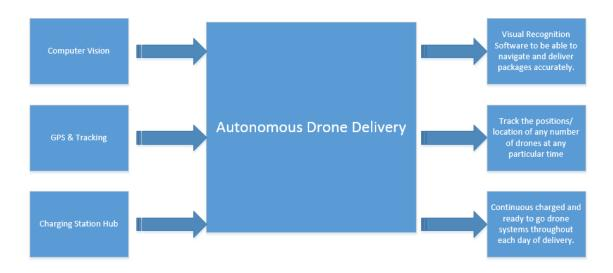
The black box diagram for the quadcopter is quite straightforward. The drone uses a combination of computer vision and GPS tracking to navigate the obstacles in front of it in order to deliver the package to the desired destination. The drone charges back at its home base on the delivery truck via the charging station hub.
