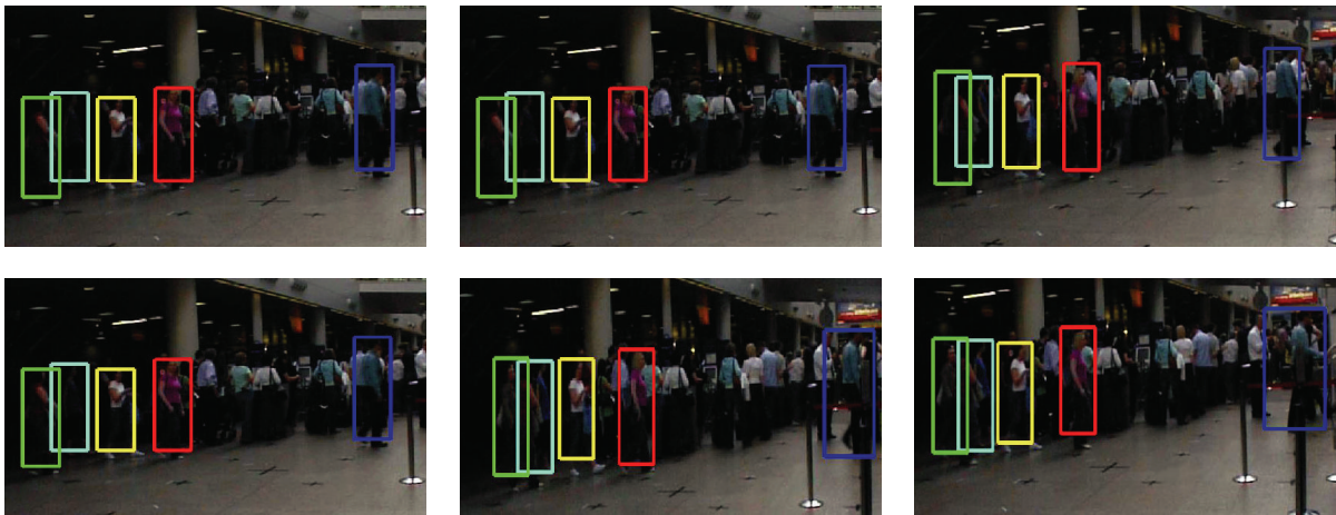
FIGURE 4: Sample results of tracking 5 targets using GMM-KL appearance model.
