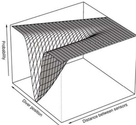
Fig. 5. Probability of detection at all positions between two sensors for various different sensor separation distances. Optimum sensor separation is that distance for which the central minimum is equal to the minimum desired probability of detection at any point.
