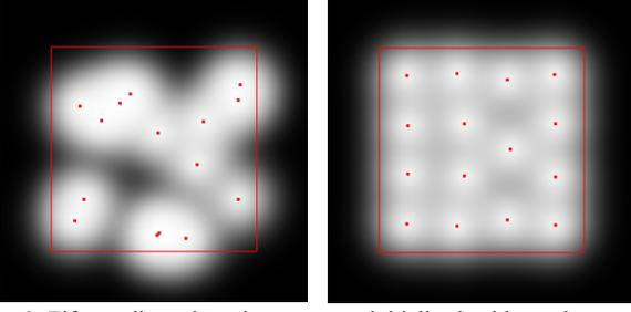
Fig. 6. Fifteen diver detection sensors, initialized with random positions (left) and after optimization (right). Square box denotes the region to be protected. Brightness denotes probability of detection. Minimum probability of detection = 0.005 (left) and 0.28 (right). Expected probability of detection = 0.67 (left) and 0.78 (right).
