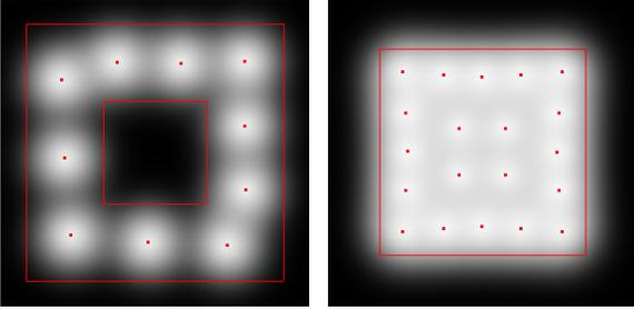
Fig. 7. Optimized sensor positions for odd shaped regions – e.g. monitoring an exclusion zone. Fig. 8. Optimal positions for 20 sensors to protect a square region. This is not a square lattice, the lines of sensors are distinctly curved.
