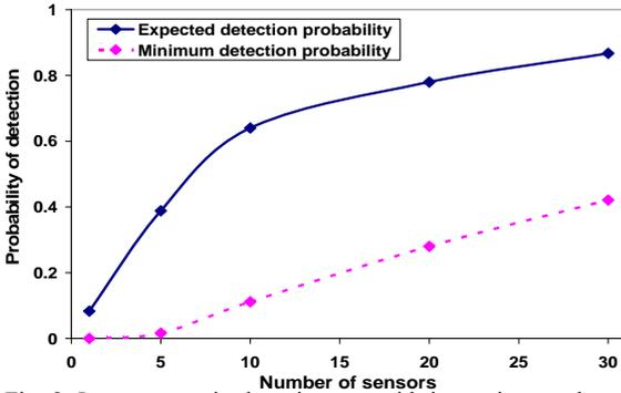
Fig. 8. Improvement in detection rate with increasing numbers of optimally positioned sensors, for the square region shown in figures 5 and 7.
