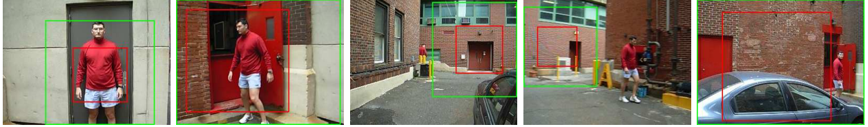
Fig. 3. Person tracking with CAMSHIFT from a moving camera in a cluttered, outdoors environment. Frames 1, 176, 735, 1631, and 1862 shown. Since the tracked person wears a red shirt, CAMSHIFT fixates on red regions of background, including brick walls and doors, and repeatedly loses the tracked person. Green and red squares indicate the search window and estimated object size respectively. This movie, PeopleTracking1CAMSHIFT.avi, can be viewed at our website[19].
