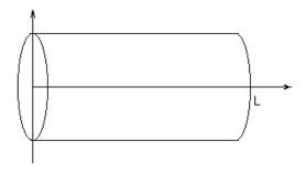
Let *u* denote the temperature in the cylinder. Suppose the ends x = 0 and x = L are kept at zero temperature whereas at t = 0 the initial temperature distribution is u = f(x). It may be shown that u = u(x, t) satisfies the P.D.E.
