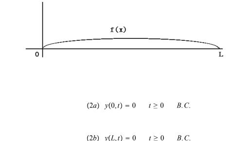
Also suppose at t = 0 string has displacement y = f(x) and is released from rest
