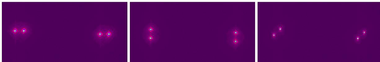
Figure 2. *Left:* FLDI legs within each bundle split horizontally; maximally sensitive to disturbances parallel with the jet flow. *Center:* FLDI legs split vertically; maximally sensitive to disturbances transverse to the jet flow. *Right:* FLDI legs split at a  $45^\circ$  angle; partially sensitive to disturbances both parallel with and transverse to the jet flow.
