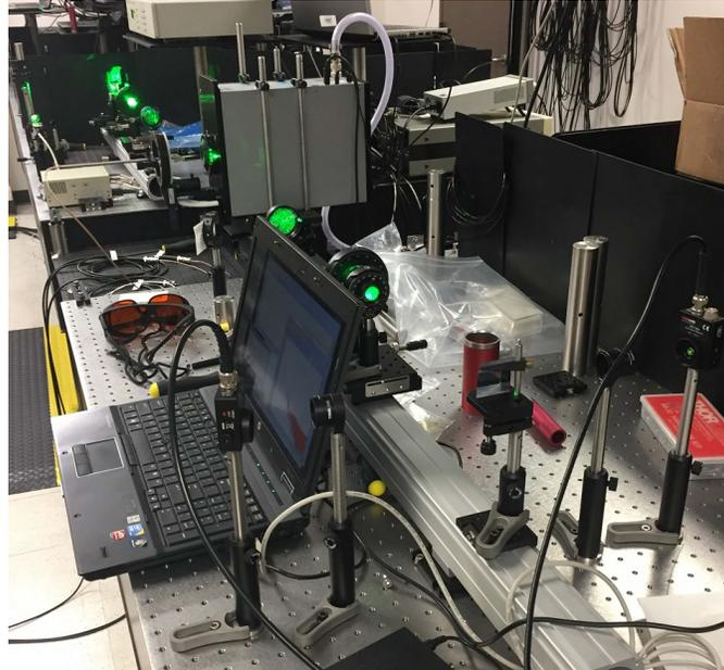
Figure 4. Dantec hotwire anemometer jet calibrator mounted across D-FLDI setup. The sensitive region of the FLDI (top left) is placed 2 mm in front of the hotwire anemometer.
