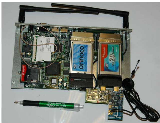
Figure 2 A GRAIL landmark that simultaneously monitors packets from WiFi, ZigBee, and Roll-Call
