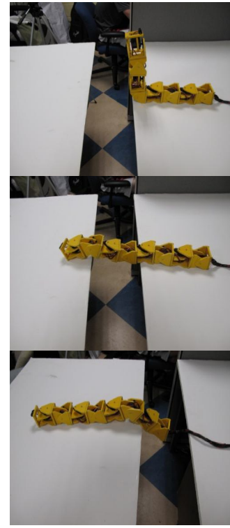
Fig. 8. The modular snake robot is crossing a gap
