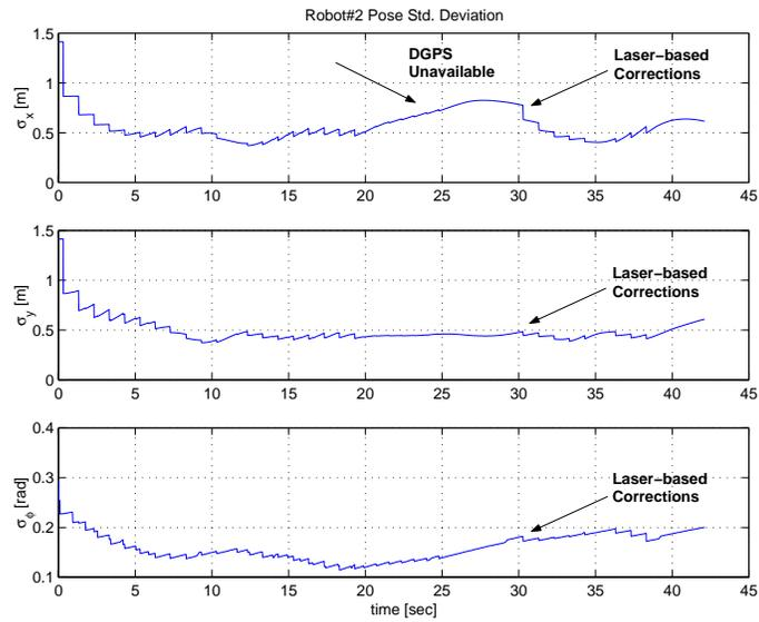
Figure 4. Laser-based cooperative localization, showing the standard deviation of the pose of robot #2. The external corrections offered by the laser-based localization scheme are marked by arrows.
