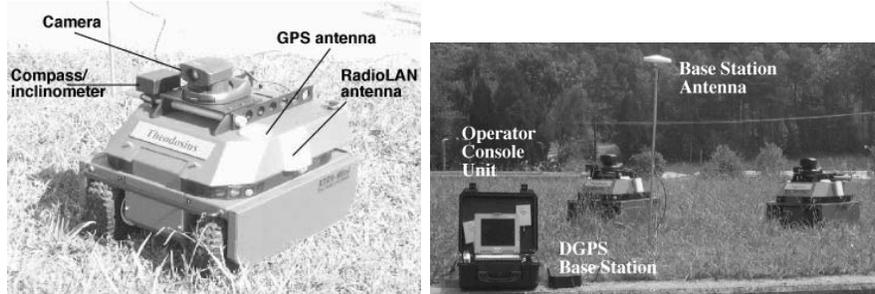
*Figure 1.* The ATRV-Mini sensor suite and experimental setup. The sensor suite consists of encoders, DGPS, a compass and a PTZ camera. The experimental setup depicted in the second photo consists of an operator console unit, a DGPS base station and a base station antenna. See text for further details.
