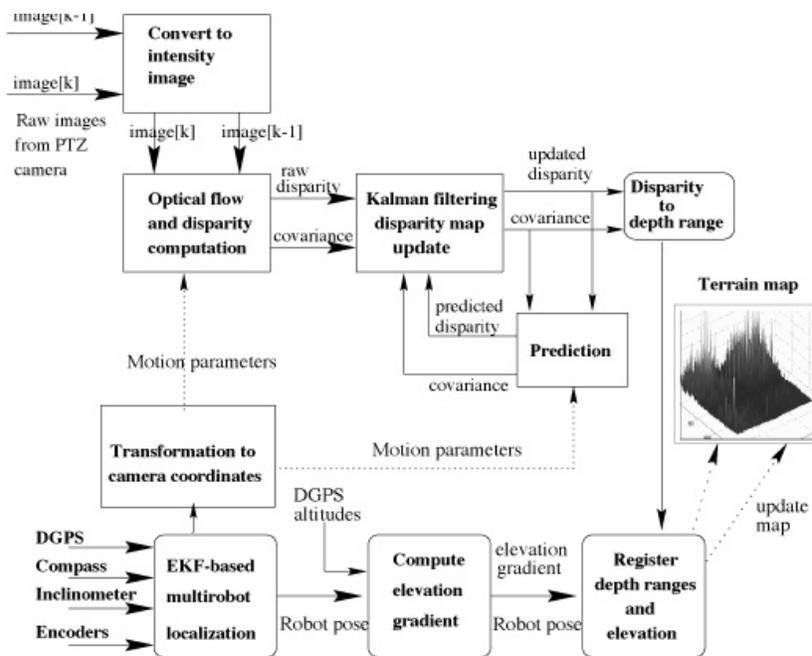
Figure 2. The overall terrain mapping scheme
