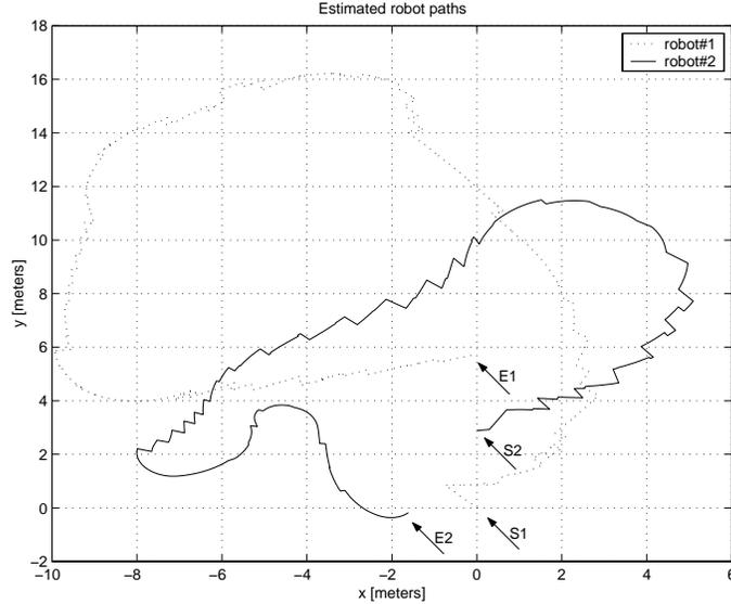
Figure 3. EKF estimated robot paths. The solid line denotes the estimated path of robot #2 and the dotted line that of robot #1. (S1,E1) and (S2,E2) denote the start and end positions for robots #1 and #2, respectively.
