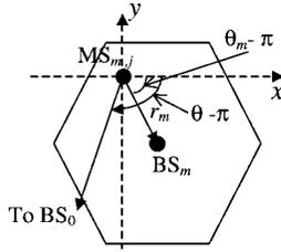
Fig. 3. Angle notations in transmit beamforming at  $MS_{m,j}$ .
