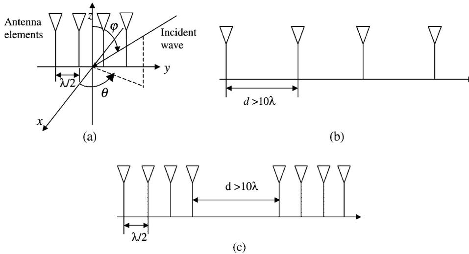
Fig. 1. (a) A linear equally spaced beamforming antenna array, (b) diversity antenna array, (c) antenna array combining beamforming and diversity.
