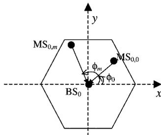
Fig. 4. Angle notations of receive beamforming at  $BS_0$ .
