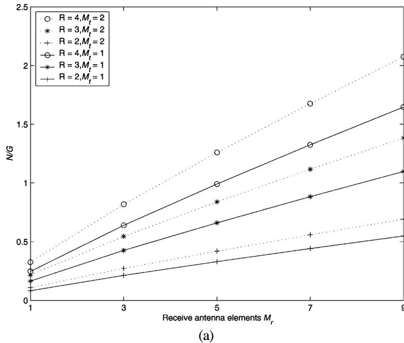
Fig. 6. User capacity, effect of beamforming and Rake receiver, (a) Uniform PDP, (b) Exponential PDP.
