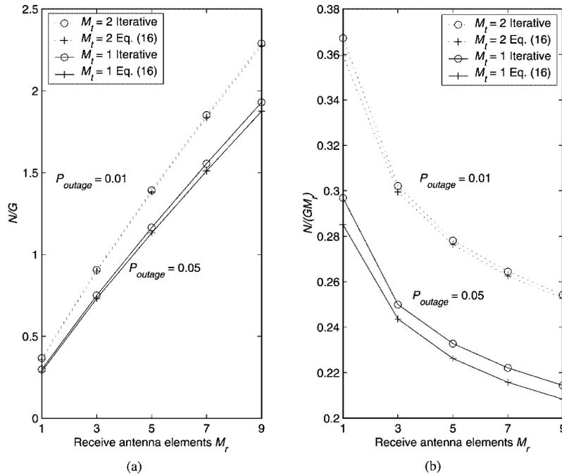
Fig. 5. Reverse link user capacity, (a) Effect of beamforming, (b) Per receive antenna element.
