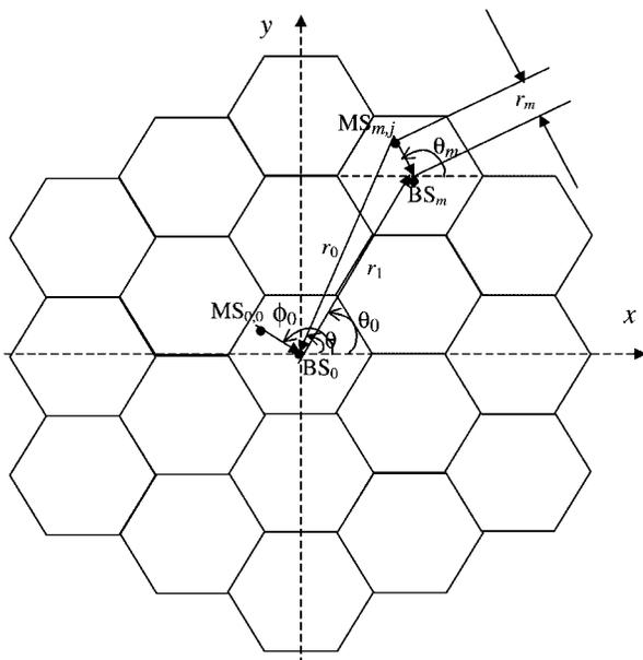
Fig. 2. Cellular structure and reverse link geometry.
