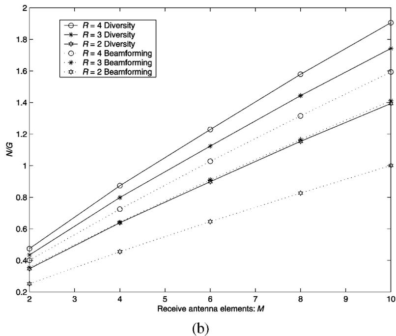
Fig. 8. Reverse link user capacity with beamforming and antenna diversity ( $d = 10\lambda$ ) (a) Uniform PDP, (b) Exponential PDP.
