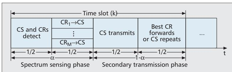
**Figure 5.** Time slot structure of the cognitive transmissions with multiple relays.
