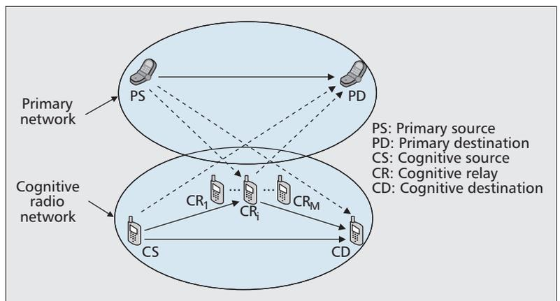
Figure 3. A cognitive radio network with multiple cognitive relays.
