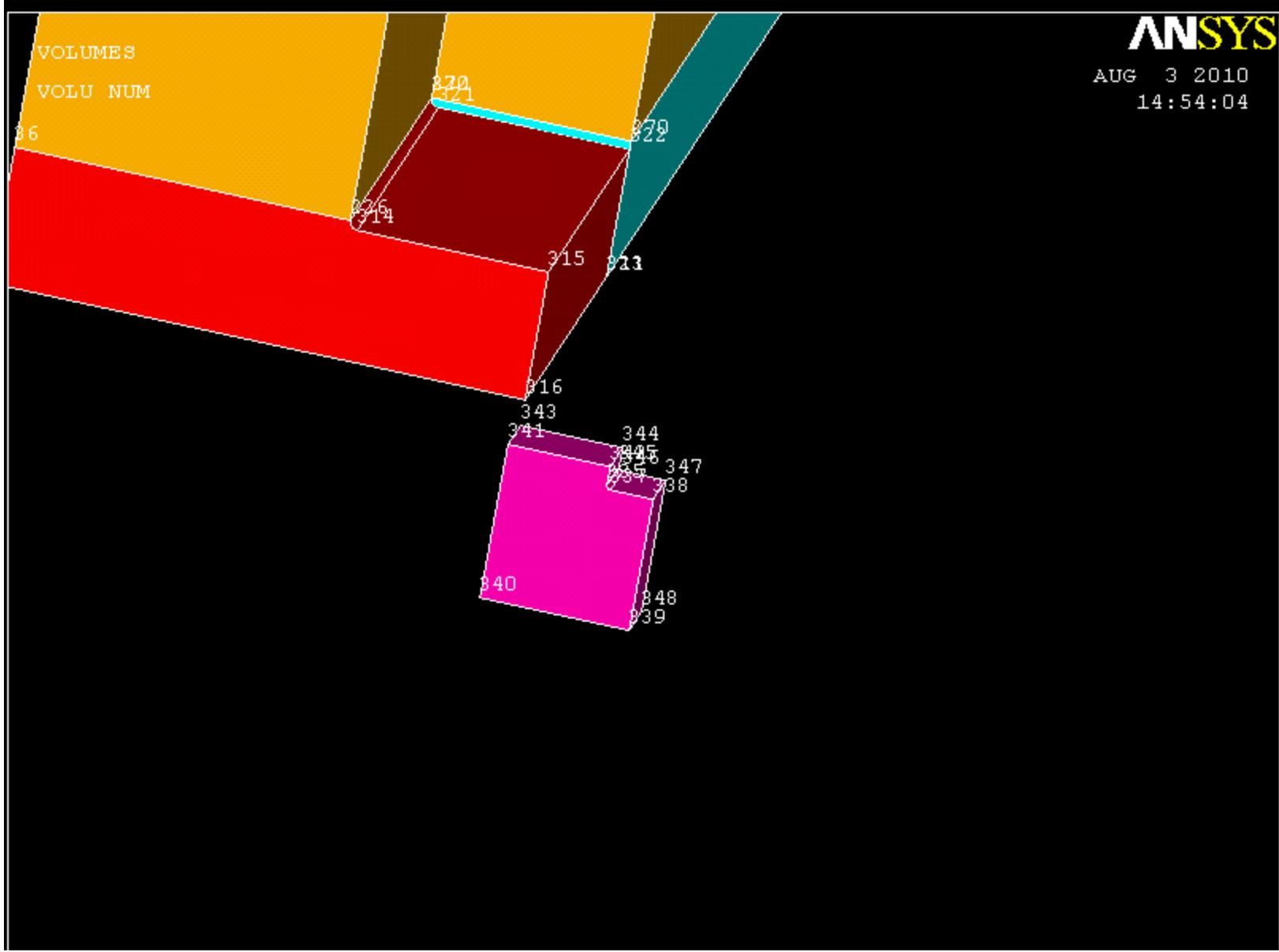
Extrude the rightmost area of the new volume .5 in the y direction
