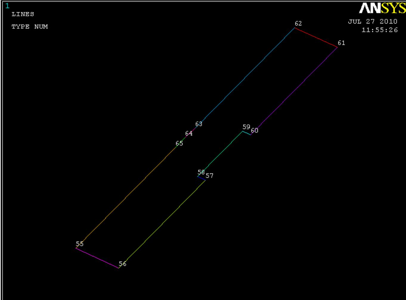
Create fillets in the inner corners by selecting (*create >> lines >> line fillet*) and picking the two lines that intersect each other to form the inner corners. When prompted for the radius type in .3125 and hit apply. Repeat the steps and hit okay to create a second fillet. Your lines should look like this:
