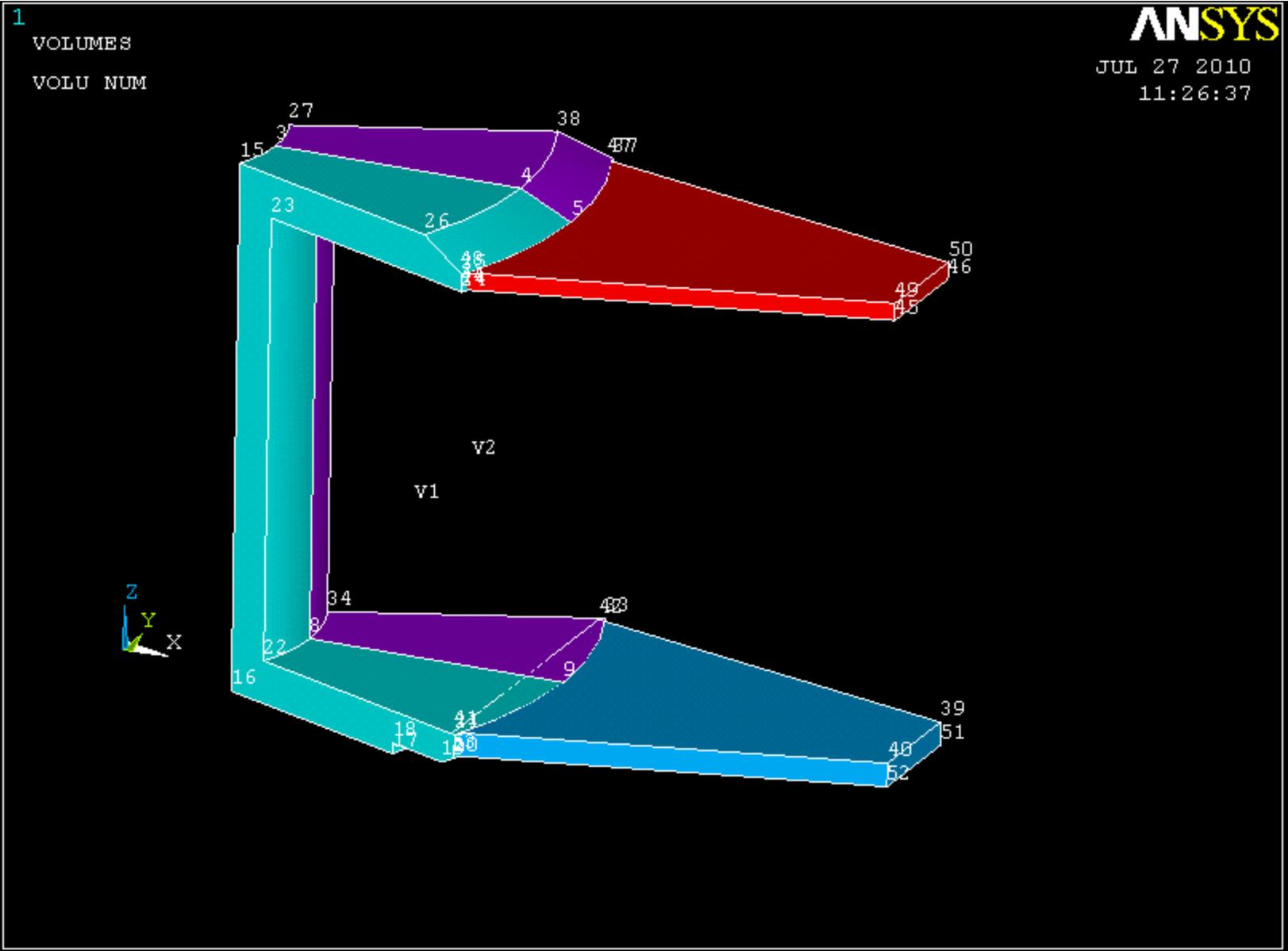
Create 11 more keypoints and connect them by lines to create the shape below. You can plot lines by typing "lplot" in the command line or clicking *(plot >> lines)*.
