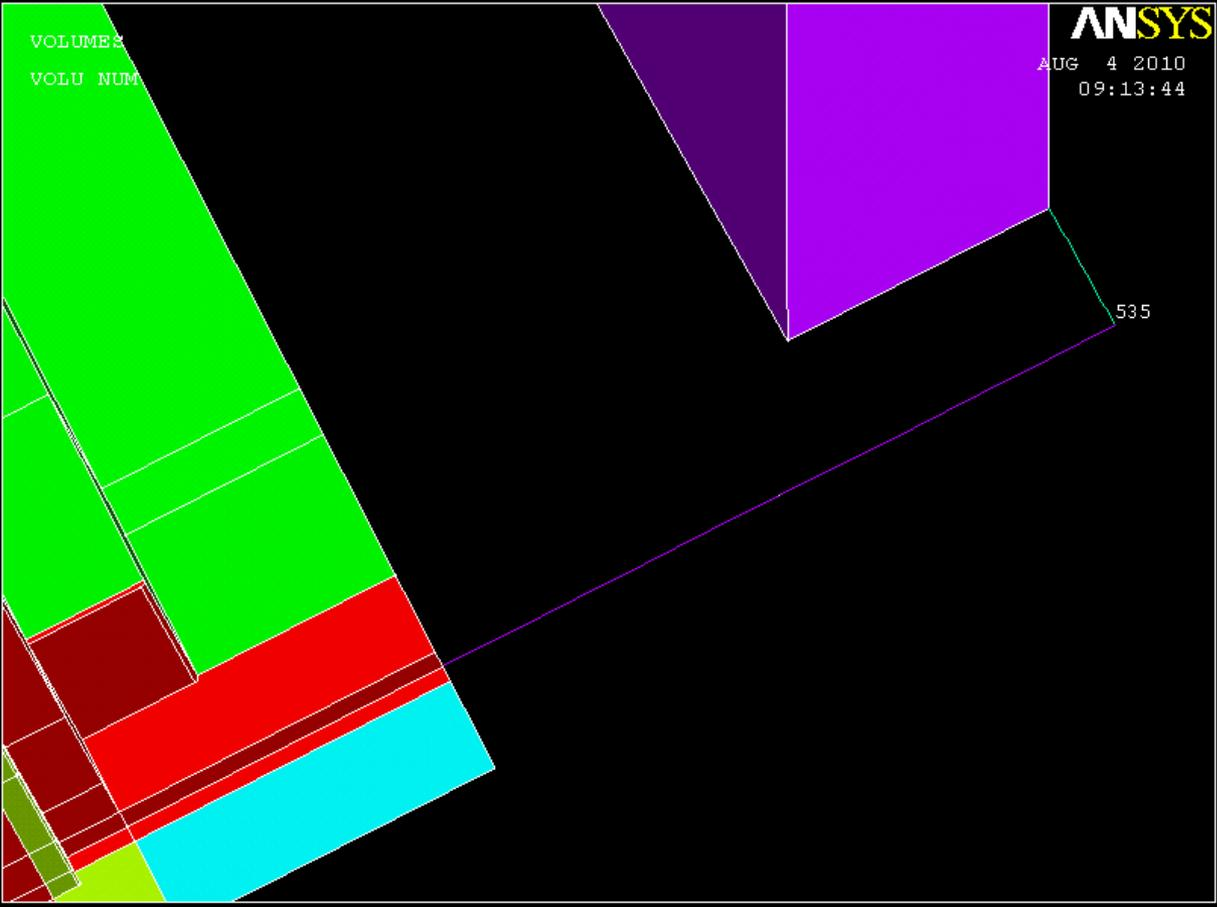
Create an area by lines. Remember the long lines on the left and right are made up of multiple lines – be sure to select them all.
