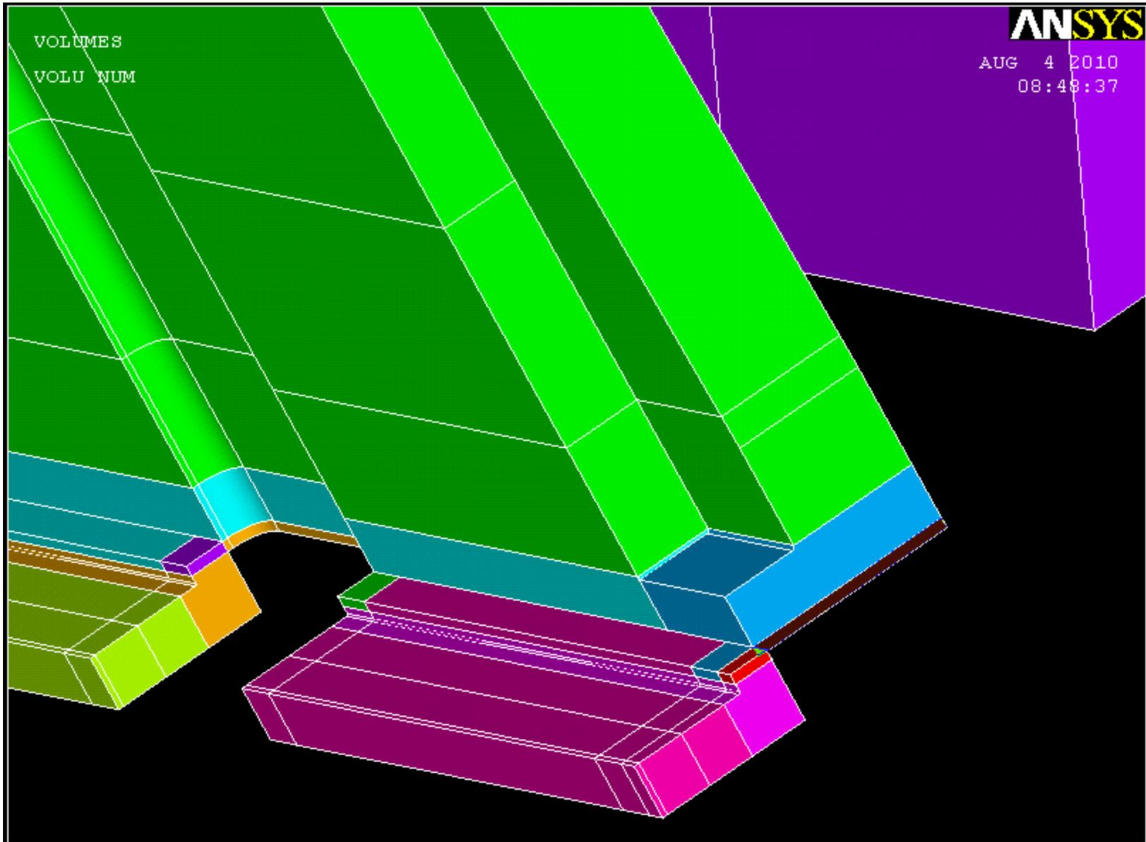
Extrude the highlighted face shown below by  $-.25$  in the  $y$  direction.
