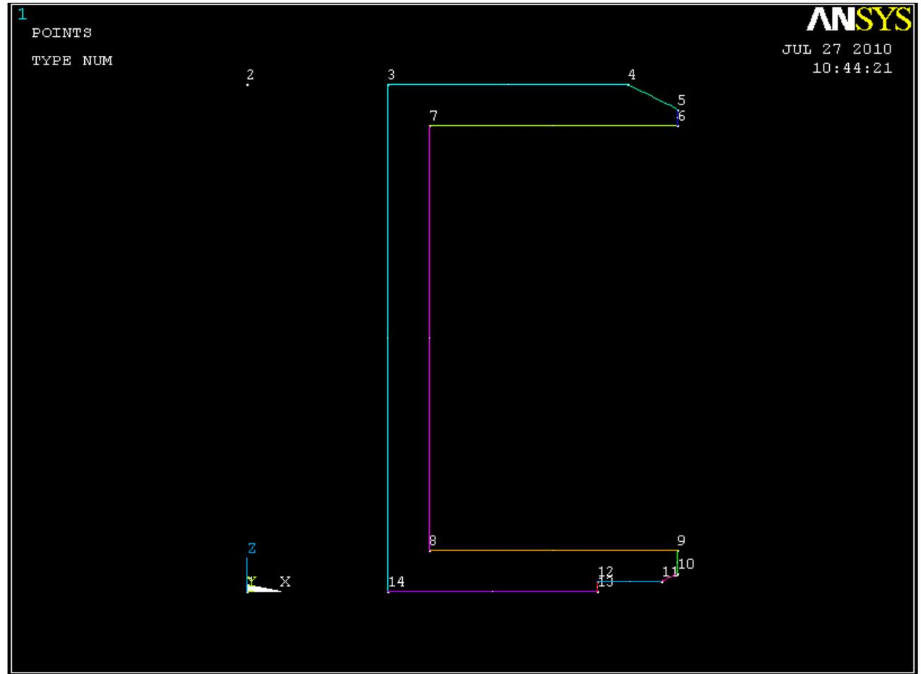
Create the area to be extruded (*creates > area > arbitrary > by lines*), when done, click okay to exit the box. Select the lines in order – start at one line and then click the one with the coincident endpoint, until you complete a closed area (ANSYS is dumb and crossing lines and keypoints confuses it). Your area should look like the one below.
