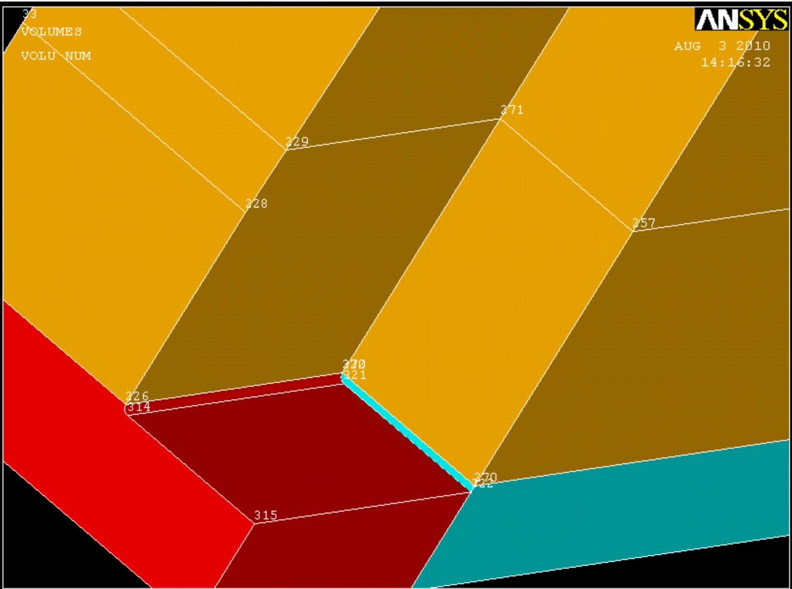
Create 5 new keypoints. Using the first (endpoint) and second (center point) keypoints, and the right most point of the second volume, create an arc of radius .03125. Connect the rest of the new keypoints with straight lines to form the area below.
