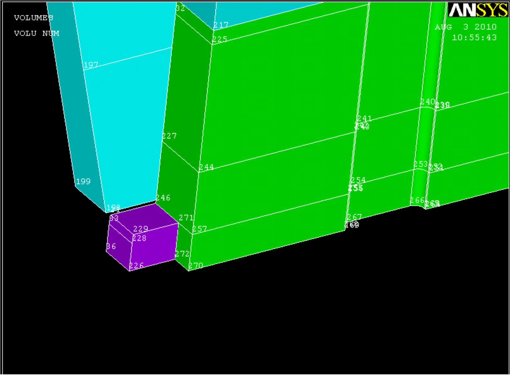
Create 3 keypoints. Then create an area by keypoints as shown below. Create an area by keypoints and extrude the area 1.25 in the X (same volume created opposite side)
