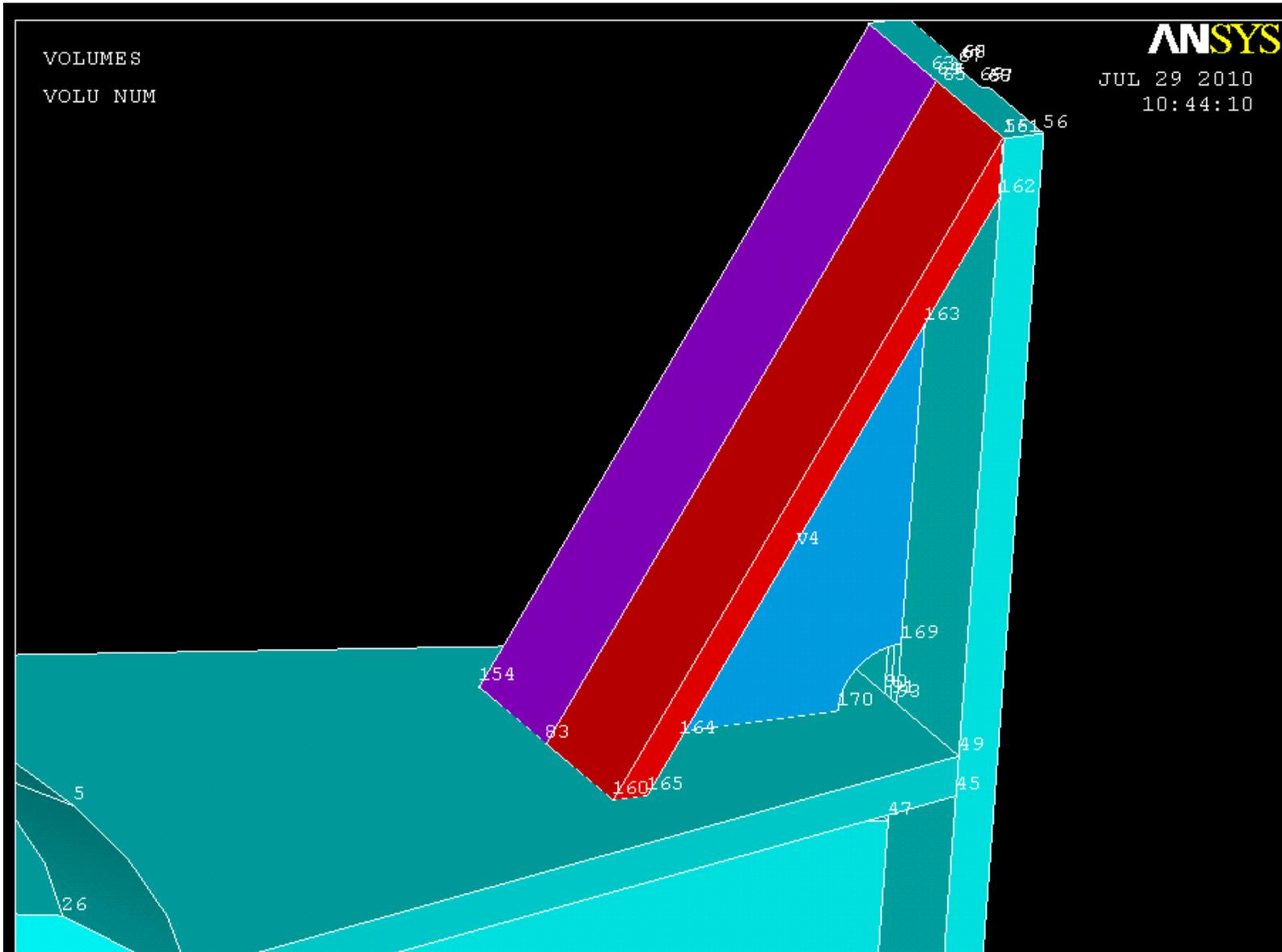
Create 6 new keypoints. Connect them with 6 new lines as we did in the last set. Then create an area by lines. The arcs and extra lines should be used for reference for the next slide's instructions – in other words I forgot to take a screenshot.
