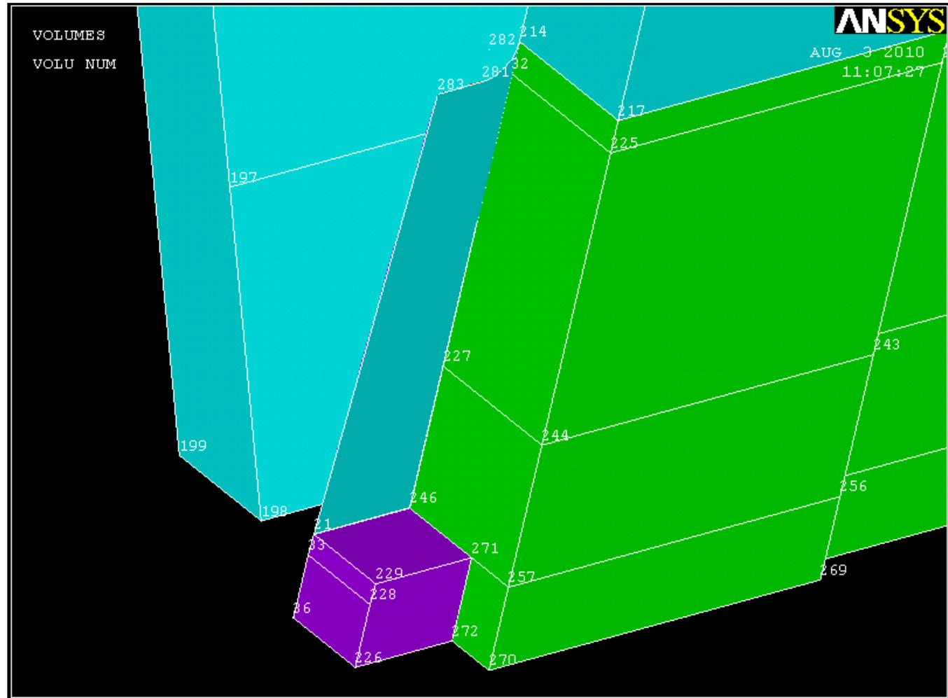
Create 3 keypoints. Using the first two and the keypoint that intersects both volumes create an arc of radius .5 (the first keypoint listed and the keypoint on the body are the end points and the second keypoint listed is the center). Connect the last keypoint listed and the to the end of the arc and to the volume below it using straight lines, then create an area by lines as shown below. Note: the vertical line is actually 3 lines vertical lines when you are selecting.
