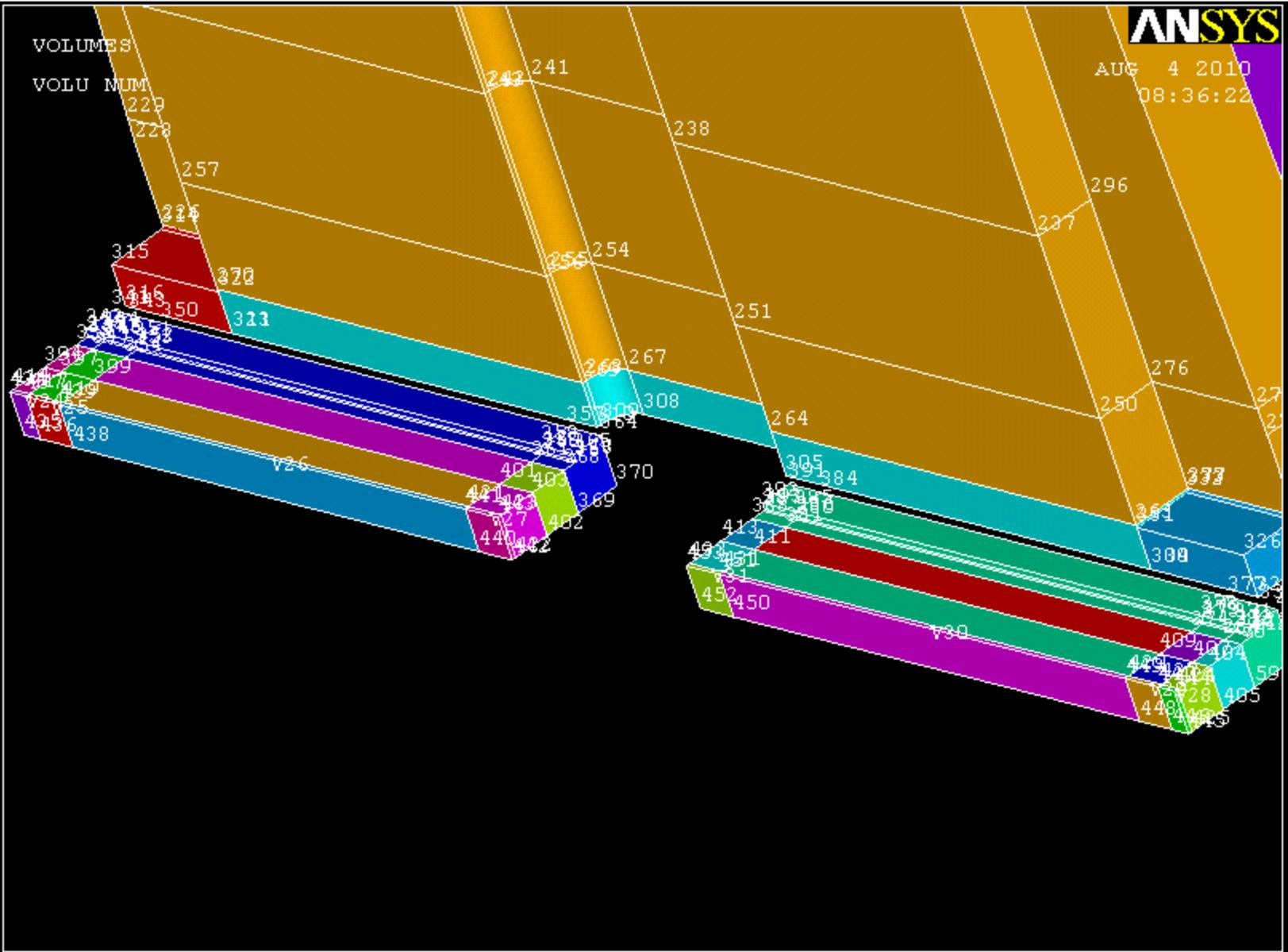
Extrude the eight highlighted faces shown below by .1 in the z direction. (Keypoint numbering has been turned off for now (*Plot Controls >> Numbering*))
