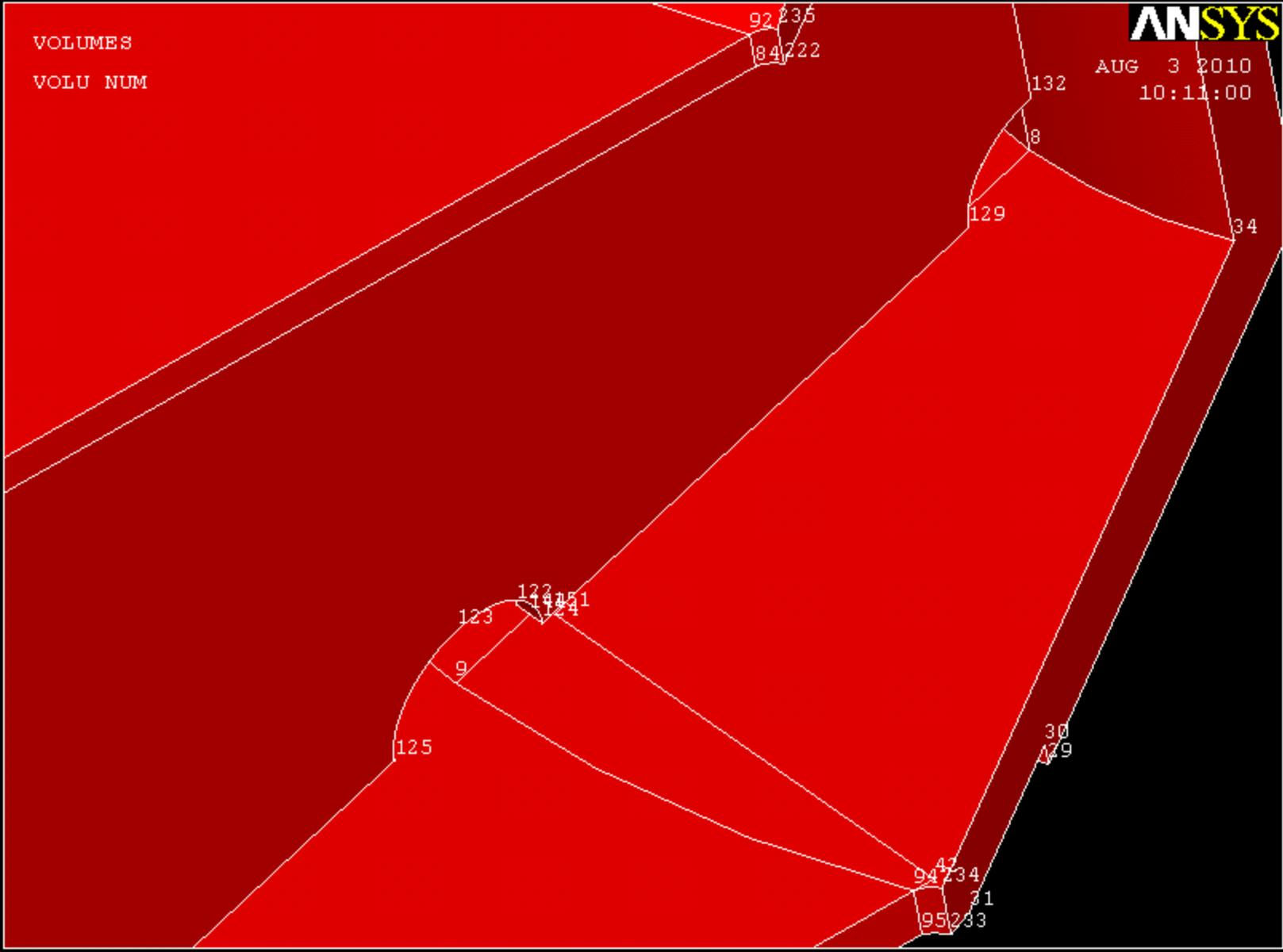
Creating keypoints without creating keypoints – this is a little trick in case you forget something or mess up. We need keypoints on the mid plate of the bottom of the spider arm. So we can extrude a face downwards, and then add and subtract to create keypoints on an existing volume. First, select this face and extrude twice, both -.5 in the z direction.
