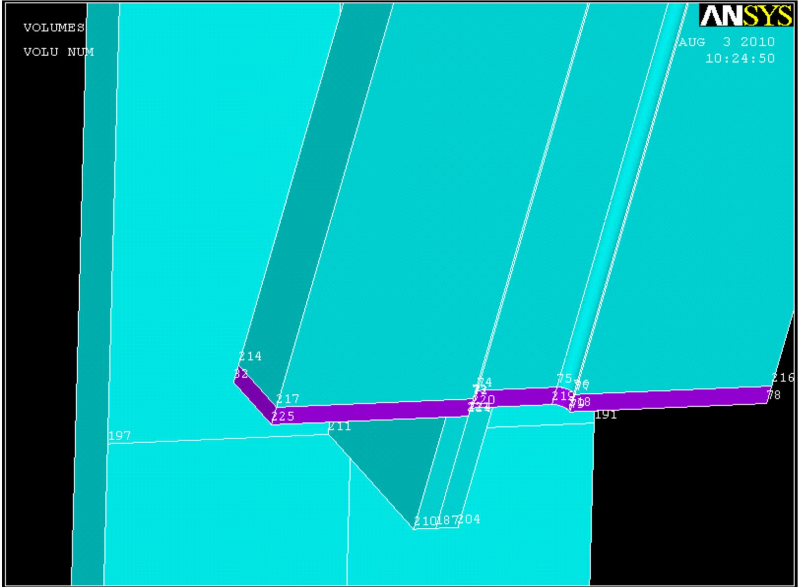
Now, extrude the bottom area of the new volume -4.5 in the z direction (again to match keypoints).
