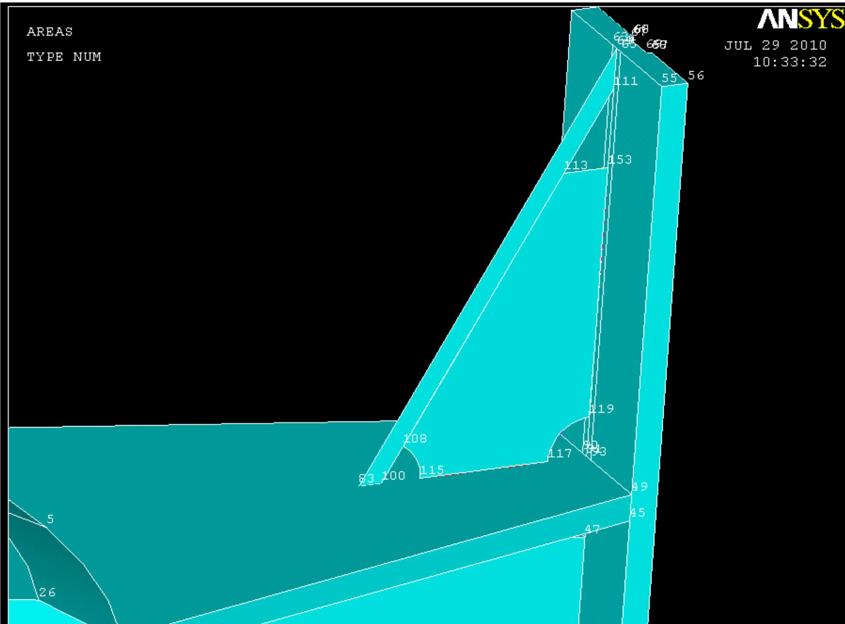
Extrude the thin area by 6.875 and -6.875 in the Y direction. Extrude the more complex area .625 and -.625 in the Y direction.
