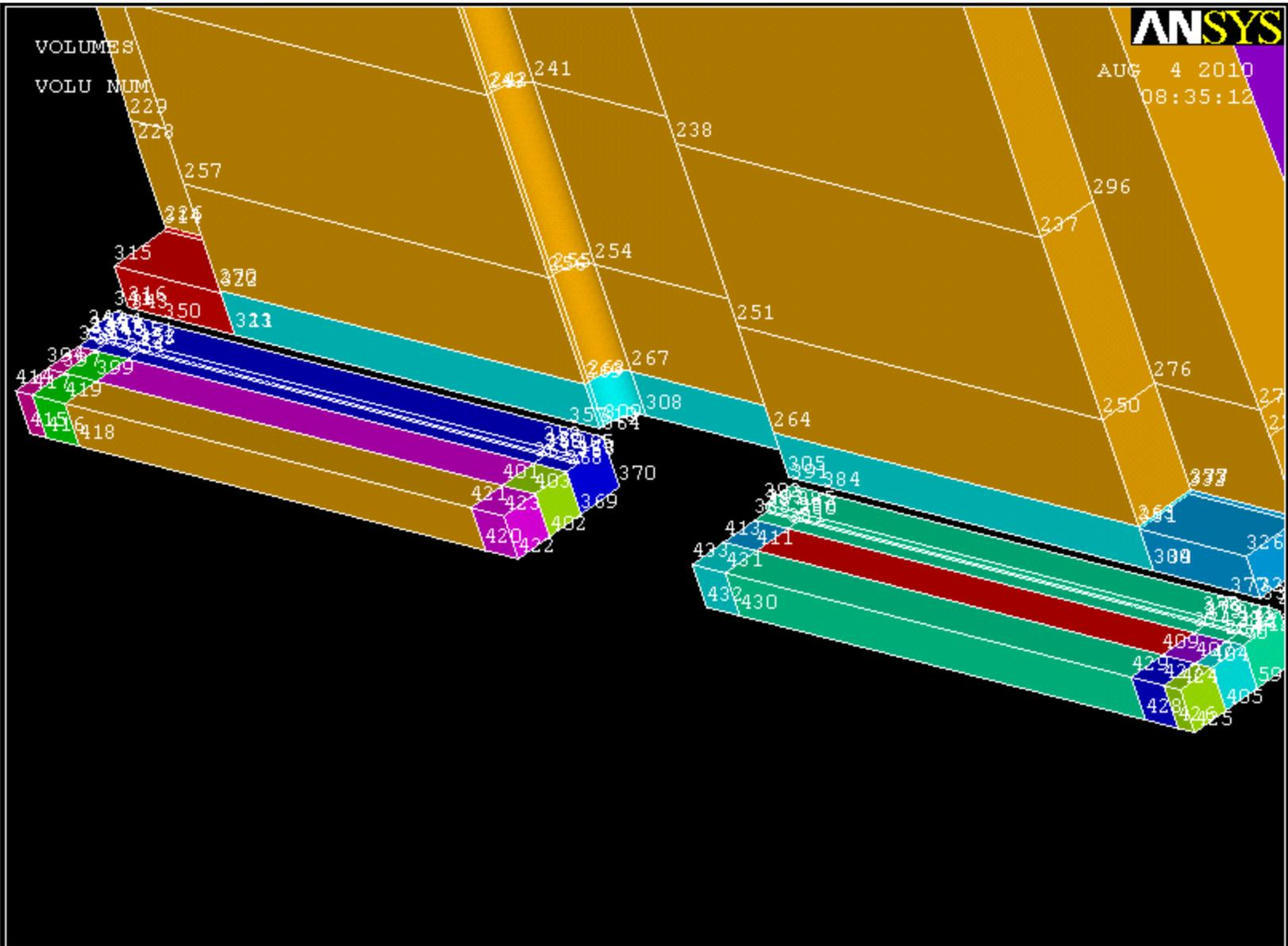
Select the front faces of the new volumes, and extrude them .05 in the x direction again (we are creating keypoints to be used for the model with the blocks later).
