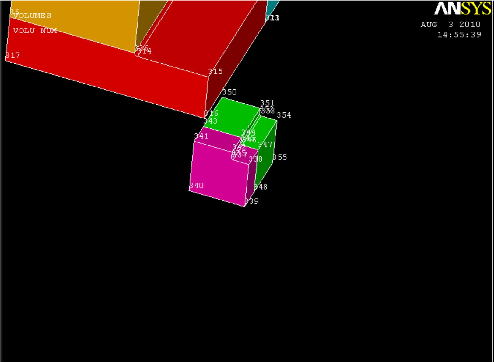
Extrude the rightmost area of the new volume 6.1875 in the y direction
