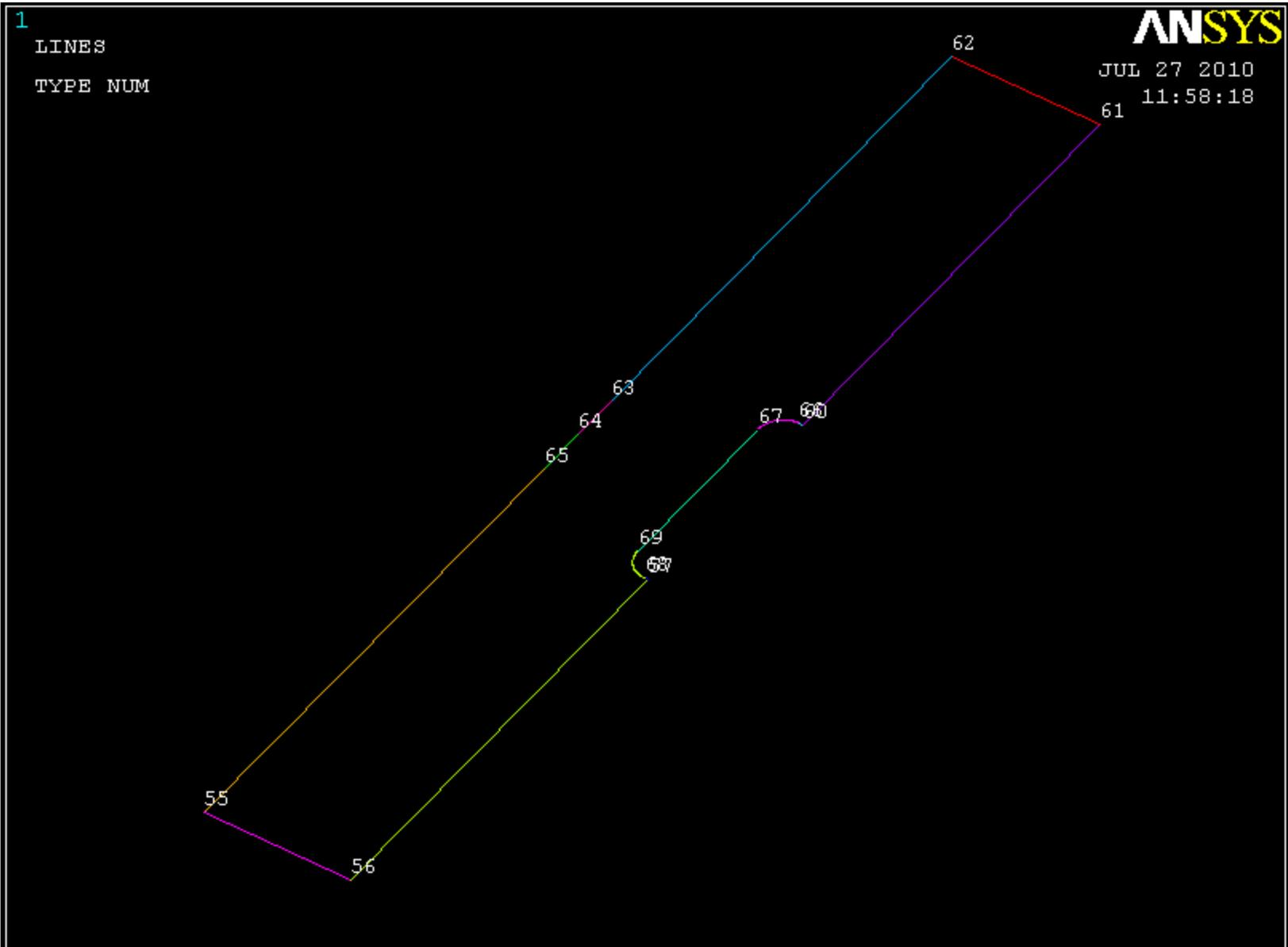
Create an area by these lines (remember the line fillet command has created 2 lines – one straight and one curved) and extrude it -107.141 in the z direction, using the “by XYZ offset command” your model should now look like this:
