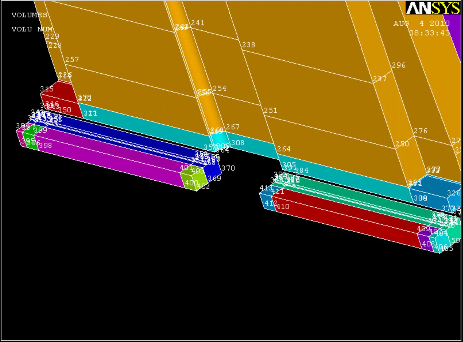
Select the front faces of the new volumes, and extrude them .45 in the x direction again (we are creating keypoints to be used for the model with the blocks later).
