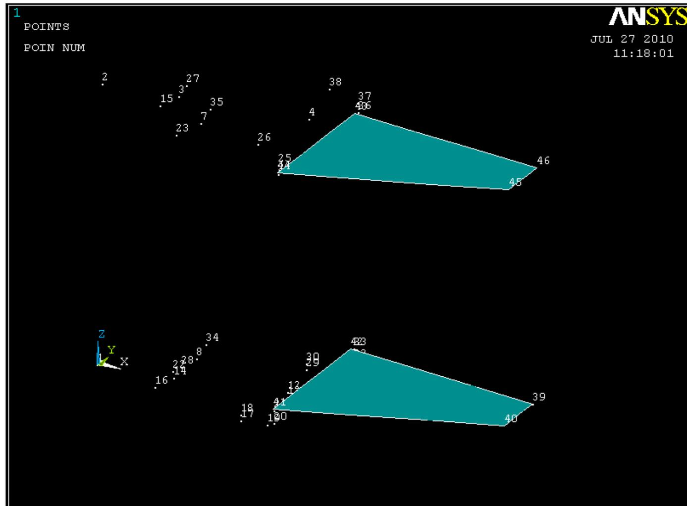
Now extrude the areas the appropriate distances - 2 for the top and -2.75 for the bottom, both in the z direction (**Operate >> Extrude >> Areas >> by XYZ offset**). To plot your volumes you can either type "vplot" into the command line, or click (**plot >> volumes**).
