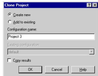
Flow Simulation now creates a new configuration. All our input data are copied, so we do not need to define our openings or goals again. The *Boundary Conditions* can be changed, deleted or added. All changes to the geometry will only be applied to this new configuration, so the old results remain valid. After changing the inlet flow rate value to 0.75 kg/s you would be ready to run again. Please follow the previously described steps for solving and for viewing the results.
