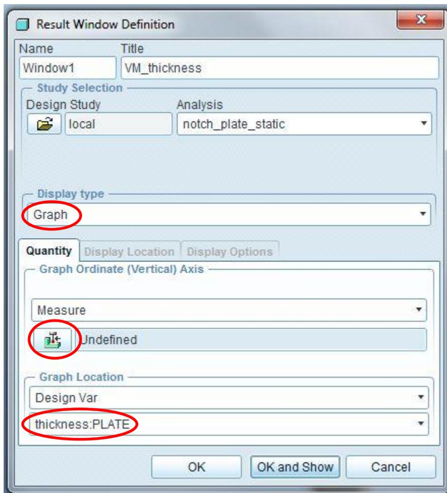
Select max\_stress\_vm as a measure and select Design Var from the graph location, make sure that the thickness variable has been selected
