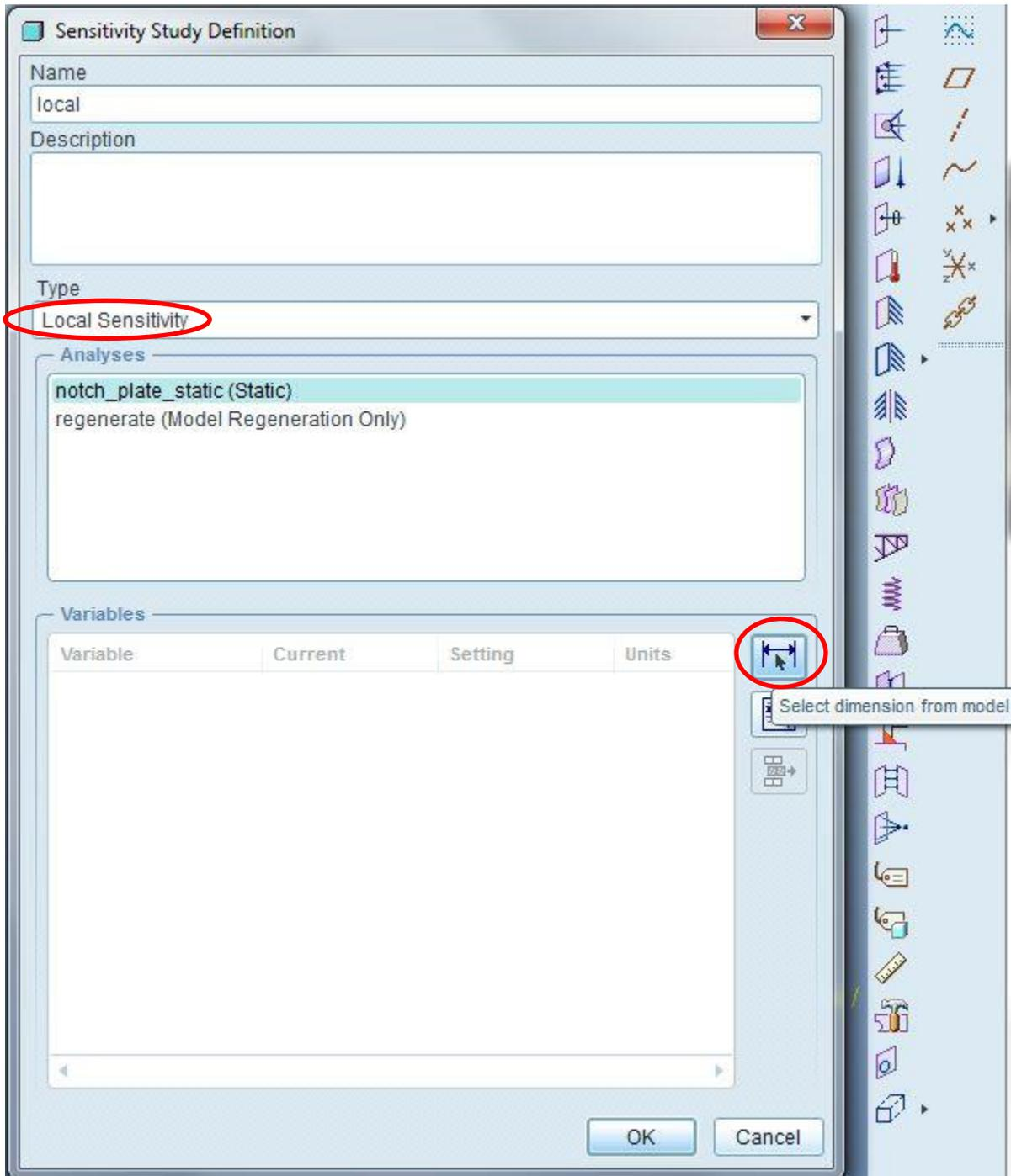
Click on the model and select the cut (notch). Select the 0.25 radius of the cut and enter the text shown below.
