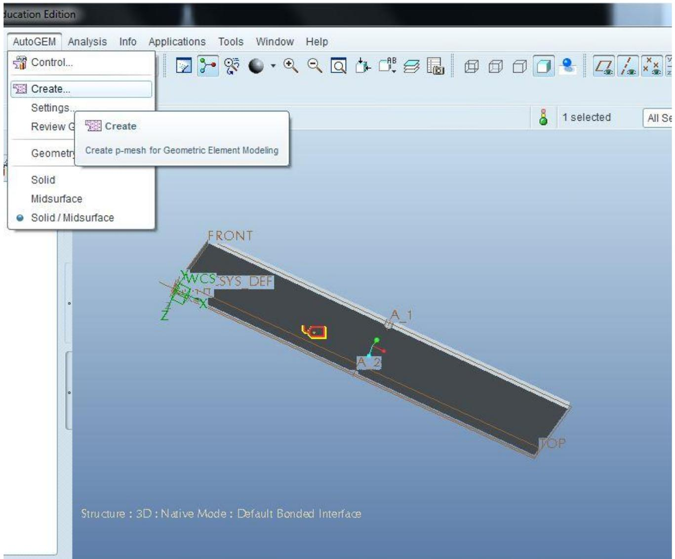
**AutoGEM**:- This command can be used to review the mesh before running any analysis. The advantage of using AutoGEM is that if the model fails to create elements after performing AutoGEM operation, we can identify which portion of the model was creating the problem. Please note that it is not mandatory to perform AutoGEM before running an analysis. If AutoGEM is not performed, elements are going to be created during the running of an analysis.
