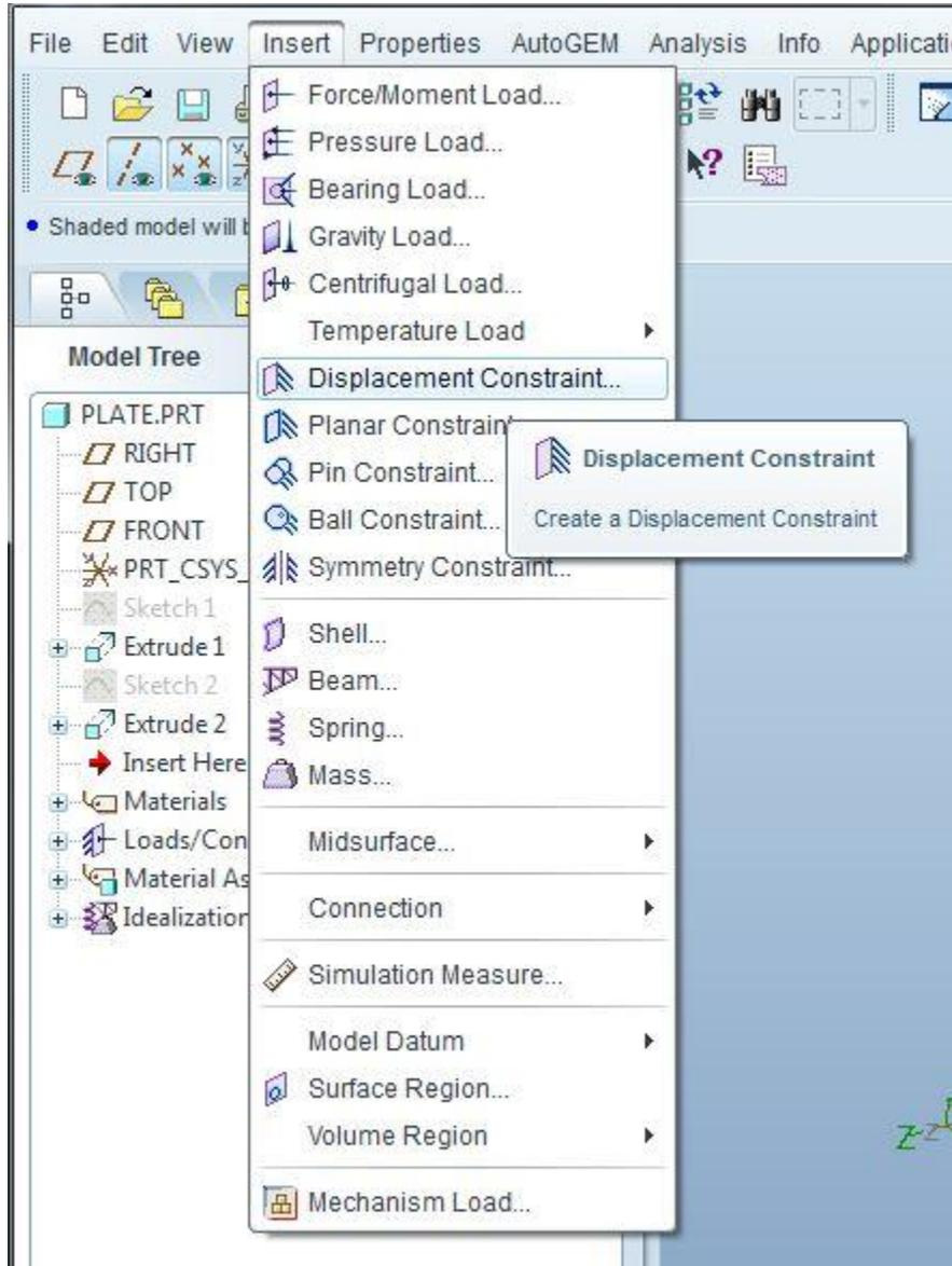
Change the name of constrains, select the edges/Curves on reference and select the left vertical edge of the model
