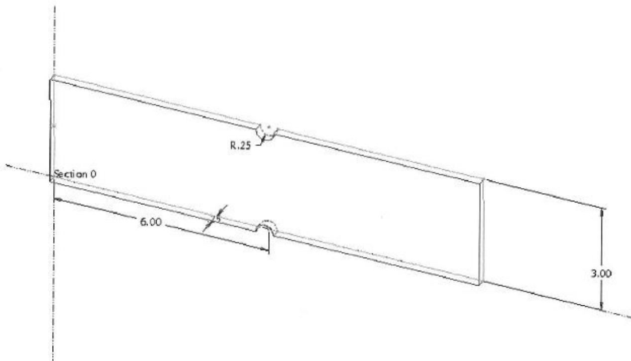
Figure 1 (Notched Cantilever Beam)
