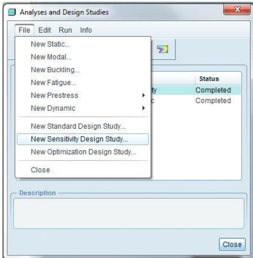
Define study name>Type **Global Sensitivity**>Select dimension from model>Select the three variables from the model>Define the start and end values of each variable as below
