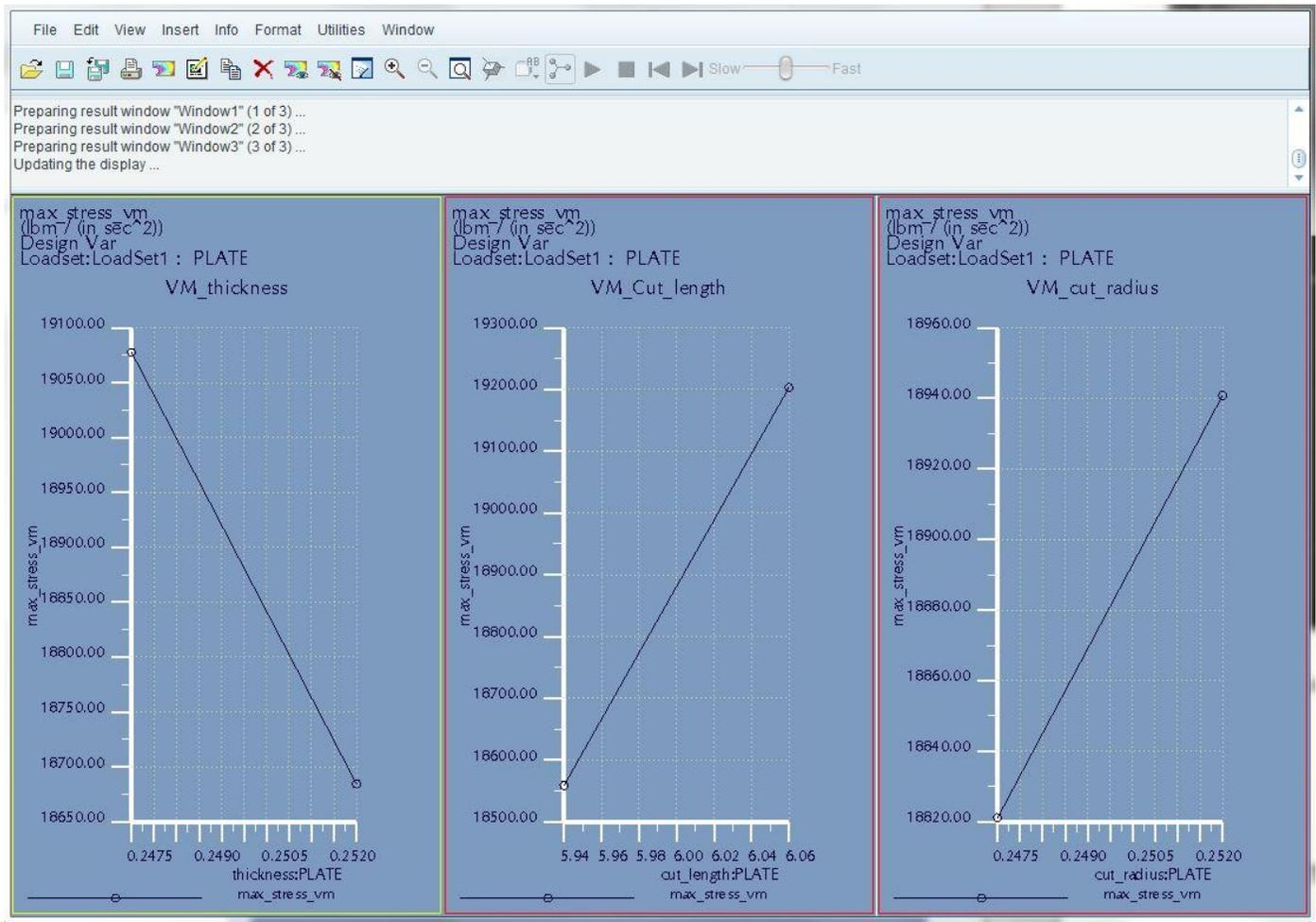
Analyze how sensitive each parameter is to the Von Mises stresses.
