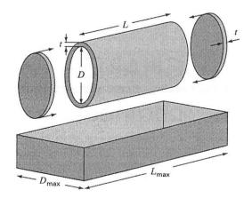
The cost consists of tank material and welding costs. Therefore, the objective function can be formulated as minimizing:
