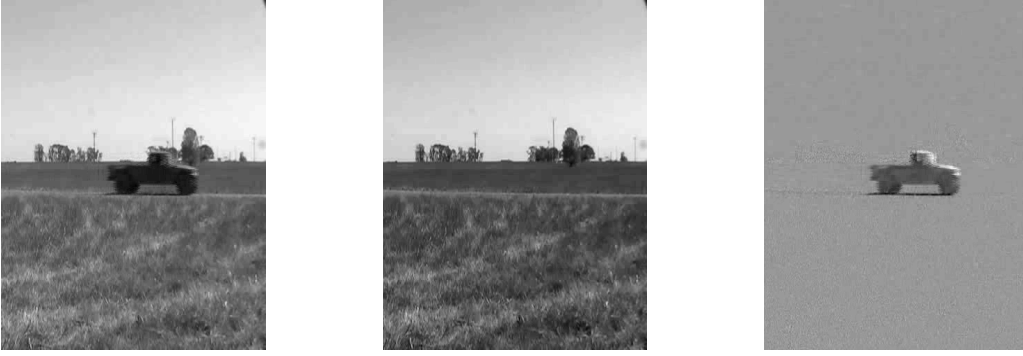
Fig. 7. From left to right: the test image x_t (40th frame of the Convoy2 data set), the background image x_b , the foreground image x_f .
