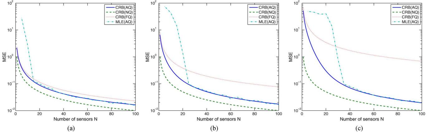
Fig. 1. CRB and MLE versus the number of sensors  $N$ . (a)  $\theta = 1$ . (b)  $\theta = 2$ . (c)  $\theta = 3$ .
