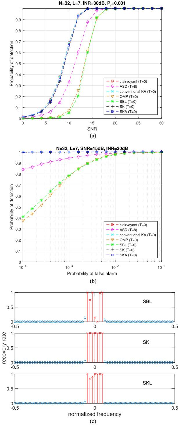
Fig. 1. Case 1 results. (a)  $P_d$  vs. SNR with  $\text{INR} = 30\text{ dB}$  and  $P_f = 10^{-3}$ . (b) ROC curve with  $\text{SNR} = 15\text{ dB}$  and  $\text{INR} = 30\text{ dB}$ . (c) Recovery rate vs. normalized frequency, with red 'x' markers indicating the locations of the true subspace bases and blue 'o' markers for other bases.
