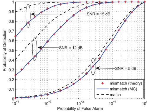
Fig. 2. ROC curves of the CFAR-MF.
