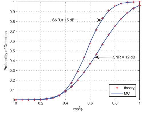
Fig. 3. Detection probability of the CFAR-MF with respect to  $\cos^2\phi$ .
