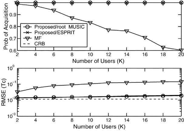
Fig. 2. Performance versus user capacity  $K$  when  $N = 16$ ,  $M = 100$ , SNR = 15 dB, and NFR = 10 dB in multipath channels.
