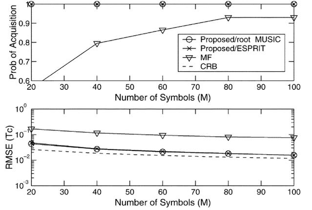
Fig. 3. Performance versus observation time  $M$  when  $N = 16$ ,  $K = 5$ , SNR = 15 dB, and NFR = 10 dB in multipath channels.
