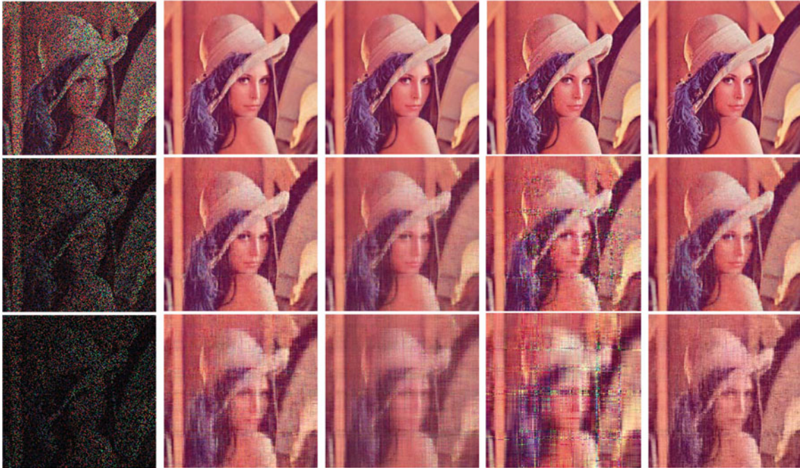
Fig. 2. RGB image inpainting. From left to right: Observed image, images reconstructed by LRTI, HaLRTC, WTucker, and IRTD. Top row: 50% missing. Middle row: 80% missing. Bottom row: 90% missing.
