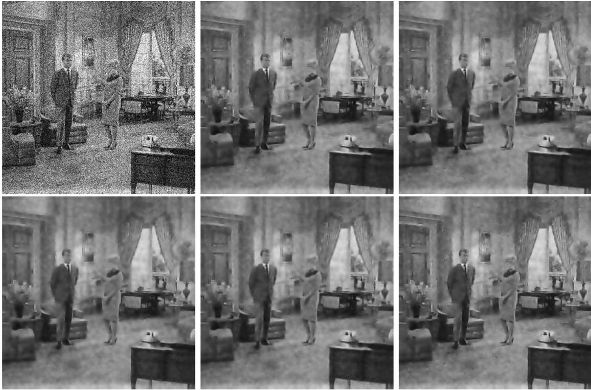
Fig. 6. Denoising results ( \sigma=50 and r=2 ) for the image "couple". From left to right: the corrupted image, the denoised image by KSVD (PSNR=24.3532 dB, SSIM=0.5918), BPFA (PSNR=24.5719 dB, SSIM=0.6062), APrU-DL (PSNR=24.1901 dB, SSIM=0.5841), SBDL-VB (PSNR=24.3299 dB, SSIM=0.5906), and SBDL-Gibbs (PSNR=24.7870 dB, SSIM=0.6170).
