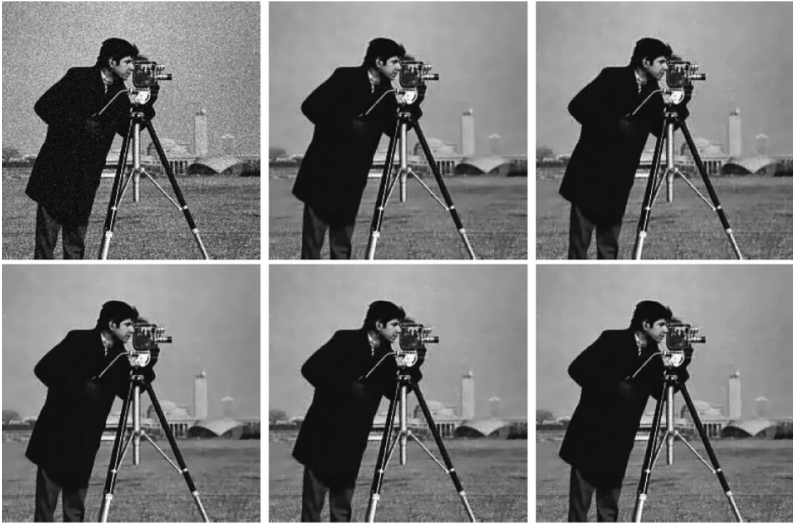
Fig. 2. Denoising results ( \sigma=15 and r=4 ) for the image “cameraman”. From left to right: the corrupted image, the denoised image by KSVD (PSNR=31.3553 dB, SSIM=0.8938), BPFA (PSNR=31.1063 dB, SSIM=0.8906), APru-DL (PSNR=31.5541 dB, SSIM=0.8952), SBDL-VB (PSNR=31.0739 dB, SSIM=0.8913), and SBDL-Gibbs (PSNR=31.4931 dB, SSIM=0.8968).
