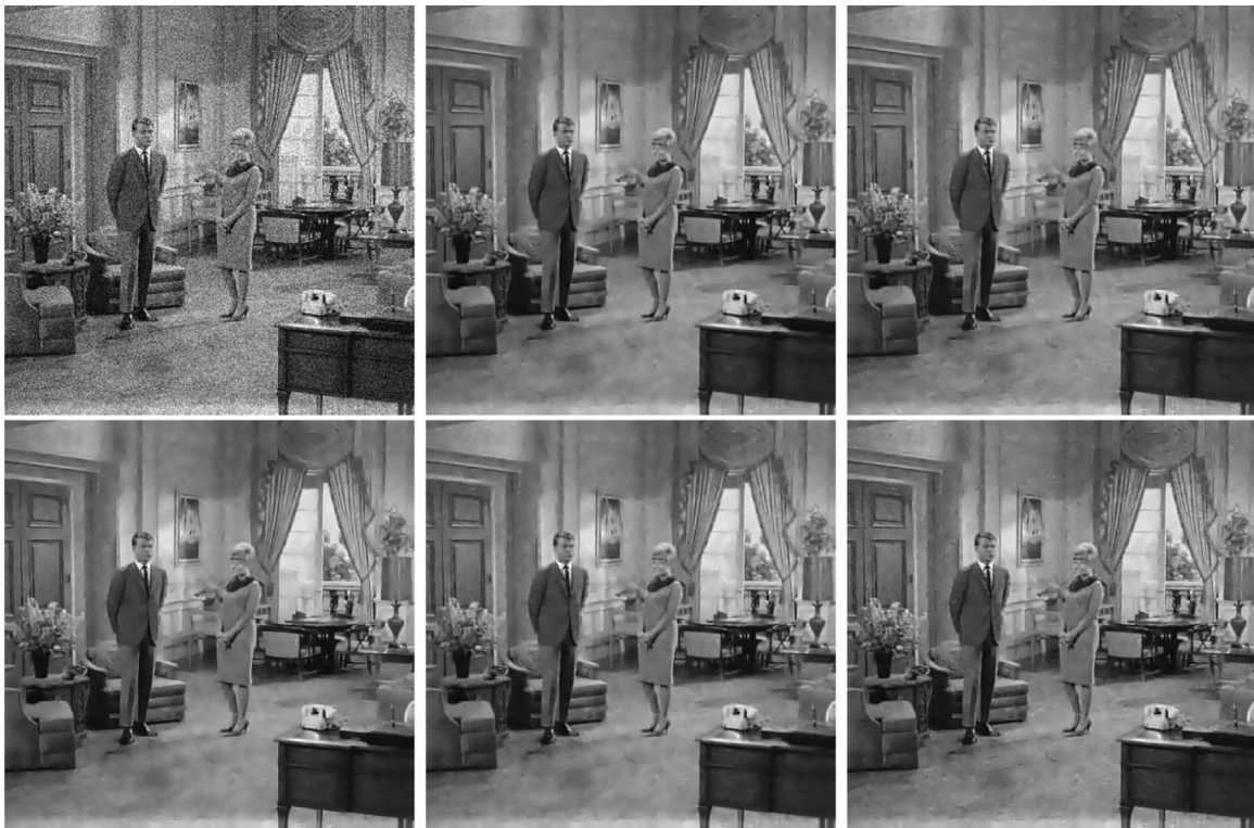
Fig. 5. Denoising results ( \sigma=25 and r=2 ) for the image "couple". From left to right: the corrupted image, the denoised image by KSVd (PSNR=28.6949 dB, SSIM=0.7710), BPFA (PSNR=28.5825 dB, SSIM=0.7735), APru-DL (PSNR=28.5378 dB, SSIM=0.7640), SBDL-VB (PSNR=28.4240 dB, SSIM=0.7641), and SBDL-Gibbs (PSNR=28.8431 dB, SSIM=0.7813).
