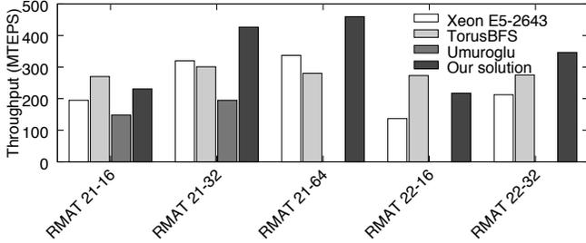
Figure 4: Comparing our design against state-of-the-art projects, i.e., TorusBFS [9] and Umuroglu [10].
