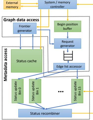
Figure 2: An overview of the accelerator design, where the green and yellow boxes are on-chip and external memory, respectively. The yellow and blue lines are external memory data and on-chip data flows, respectively.
