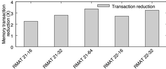
Figure 7: Reduction in memory transaction from coalesced graph data access.
