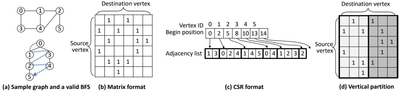
Figure 1: A (a) Sample graph, and its (b) Matrix format, as well as (c) CSR format. And (d) Vertical partition is adopted by this work for better cache designs.
