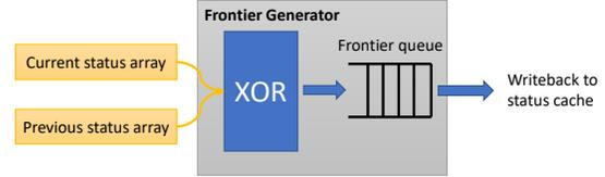
Figure 3: A detailed representation of the frontier finder module.
