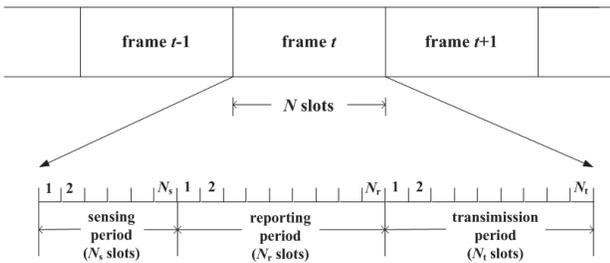
Fig. 2. Frame structure.
