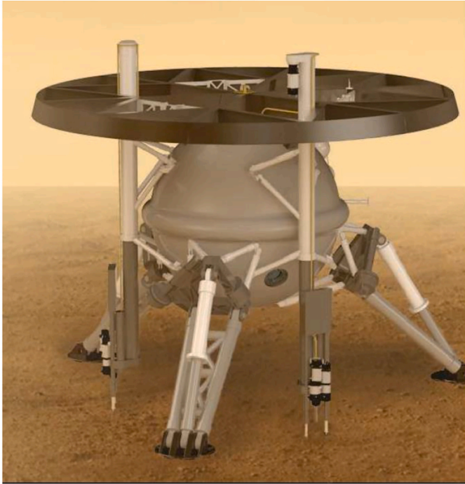
Fig. 4. A conceptual design for a Venus lander mission concept, showing a central pressure vessel with a ~1.2 m diameter, a leg footprint of diameter ~4.0 m, and a rock clearance (post-landing event) of ~0.35 m (vertical clearance between the bottom of the pressure vessel and the ground).
