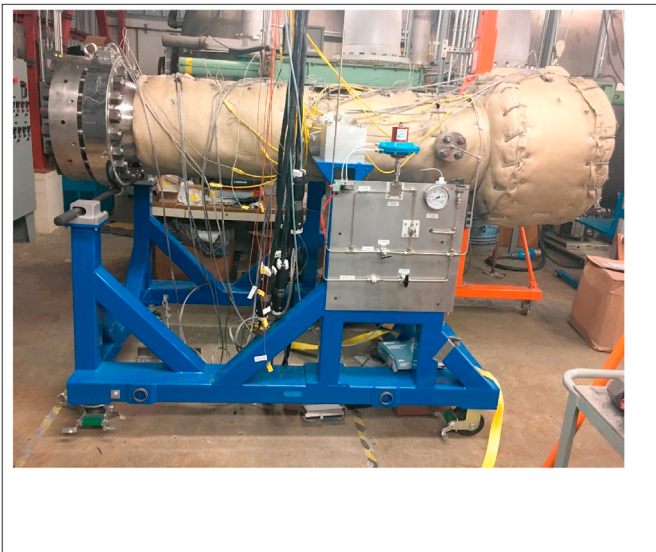
Fig. 7. The JPL Large Venus Test Chamber in the horizontal orientation. The chamber is connected to the blue frame that allows for rotation between the horizontal and vertical positions. Gas injection and venting is controlled through the silver panel in the foreground. Thermal insulation has been temporarily removed from the left flange.
