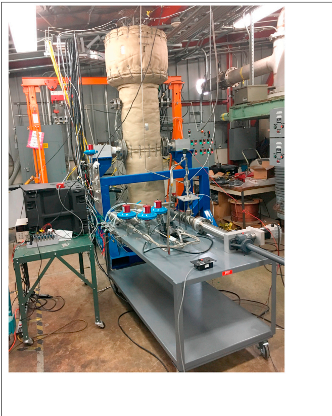
Fig. 5. Laboratory setup showing Large Venus Test Chamber (covered in white insulation) and pneumatic plumbing system.
