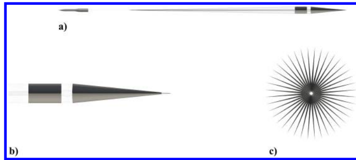
Fig. 4 Initial configuration of the FE structural model prescribed for each performed numerical FSI simulation: a) zoomed-out side view, b) zoomed-in side view, and c) bottom view.
