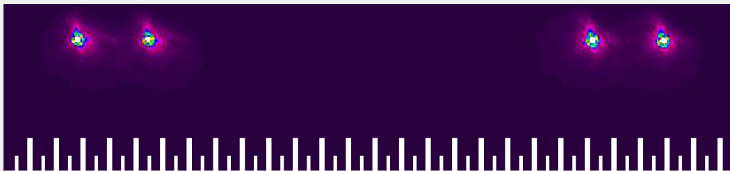
Fig. 4 FLDI beam pairs for an FLDI setup developed using diffractive optics and a 2 arcminute Wollaston prism pictured at the focus with an Ophir Spiricon LT665 beam profiler. The major tick marks are at 100 \mu\text{m} and the minor tick marks are at 50 \mu\text{m} .
